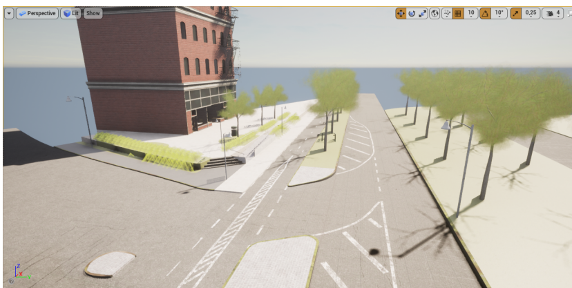
Figure 3.6: The digital model of the Lindholmen junction after it was imported into CARLA. Note that some of the signs present in figure 3.5 are missing. Some of the textures, particularly the leaves and the pavement material, also do not look particularly realistic.
