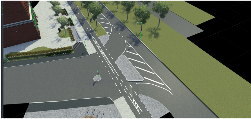
Figure 3.4: The digital model of the Lindholmen junction was created in RoadRunner. This is an image of the model. Compare with figure 3.2.
