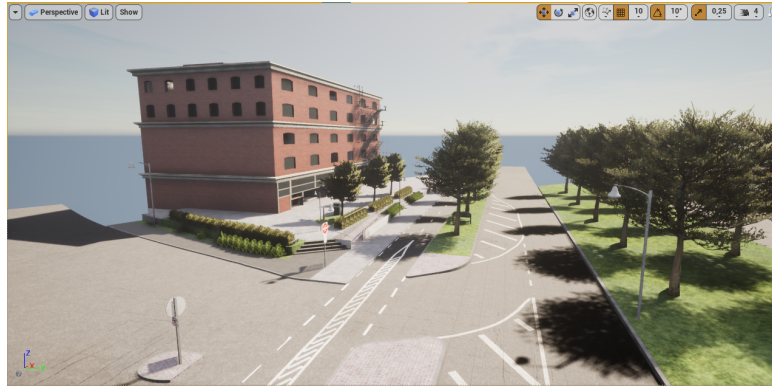
Figure 3.7: The improved digital model of the Lindholmen junction after it was imported into CARLA. Compared to figure 3.6, the tree and bush textures look more realistic, some ground material has been changed and some signs have been added. The building to the left in the image has also been re-scaled to better resemble the real one shown in figure 3.3.
