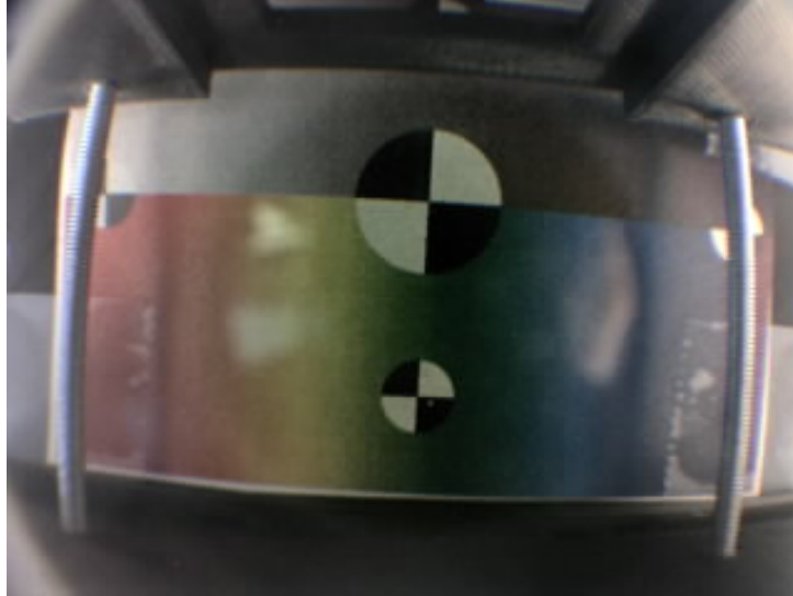
Figure 5.15: A m12 lens with a 26^\circ angular field of view and a minimum focus distance of approximately 1m. Two external lenses used in a reverse galileian formation. The negative lens had a focal length of -25 mm and the positive lens had a focal length of 60 mm. The entire reference image is present in the captured image, as well as a clear center of focus. Which means that it is usable for mikrodust.
