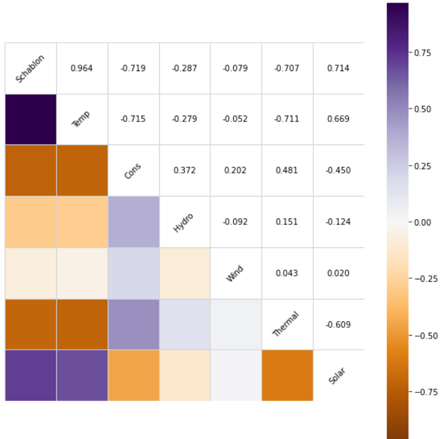
Figure 41: Correlation plot of Schablon and Swedish energy features in bidding area 1. On the diagonal we have the features examined. Above the diagonal we have the r-values, and below we have a heatmap of the correlations. From the figure we see that there's either very weak or no correlation between Schablon and wind energy ( |r| \leq 0.3 ), a moderate to strong correlation between Schablon and hydroelectric energy ( 0.5 \leq |r| \leq 0.7 ) and a strong correlation between Schablon and the other considered features ( |r| \geq 0.7 ).
