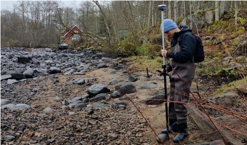
Figure 18. Bathymetric measurements were gathered in situ with a handheld DGPS.
