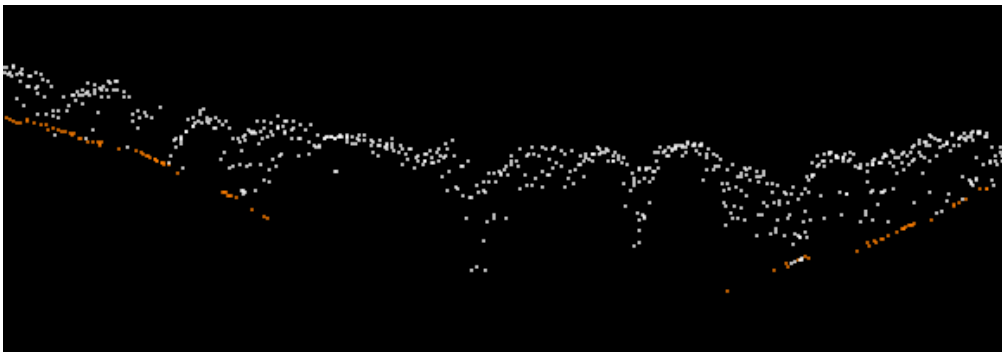
Figure 26. A dense canopy cover can block the laser from reaching the ground. Due to the shortage of ground points in the depression, the surface will be interpolated. White points are unclassified, and brown are ground (Swedish Land Survey [Lantmäteriet] 2020).
