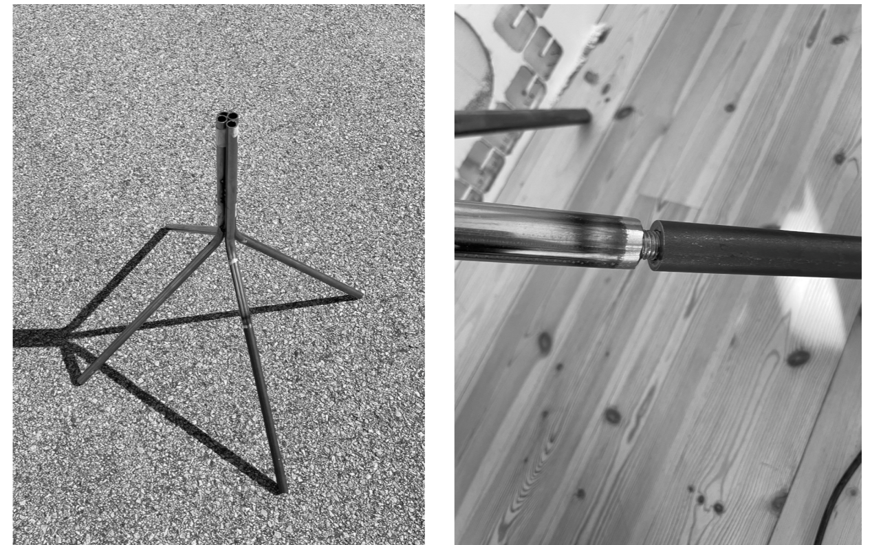
Figure 18. Mockup of levelling leg mechanism
