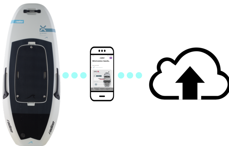
Figure 2.6: Illustration of logs uploaded from the board's internal memory and transfer the cloud via the Radinn app
