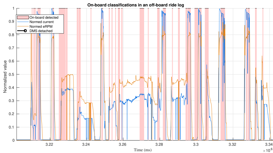
Figure 4.10: Snippet of a ride log without a surfer on-board. The red areas mark where the classifier has found an on-board window, meaning that it mistakenly thinks that a surfer is riding on the board.
