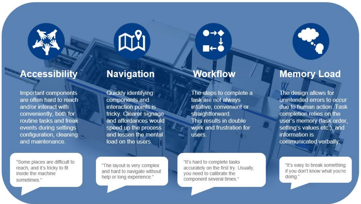
Figure 31: Main themes of the identified pain points. The themes emerged as a result from an affinity diagram of the user research input. [5]
