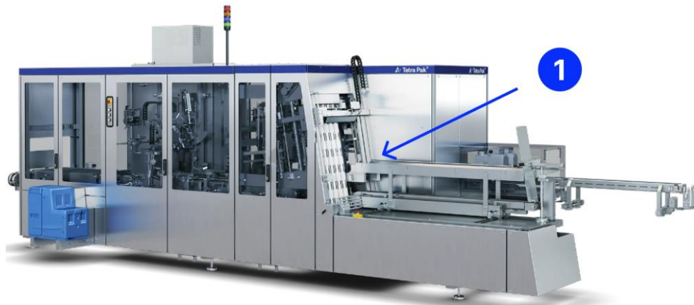
Figure 10: The Cardboard packer's tray module. The number (1) indicates the location of the carton infeed. [5]
