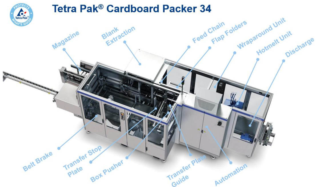
Figure 8: Overview of CBP34's main modules, split by function. [13]
