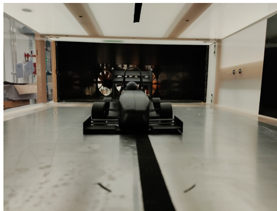
Figure 5.7: Fastening of the scaled model - Lund windtunnel
