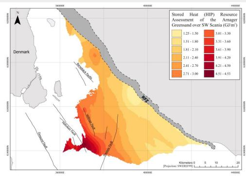
Additional deep drillings are needed to better determine the spatial distribution of the Arnager Greensand which would improve the geothermal assessment.
