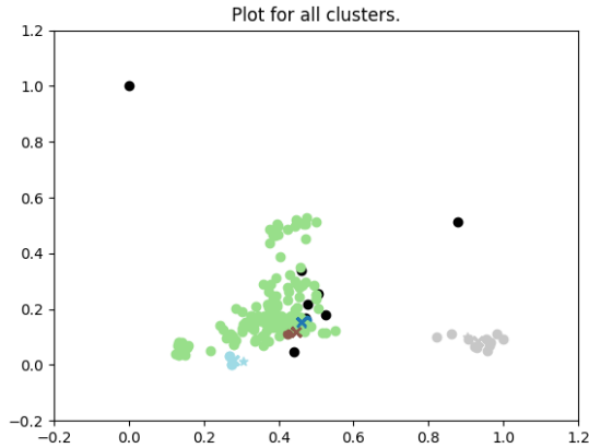
Figure 5.14 The figure shows a scatter plot of the DBSCAN clustering with the highest coverage in relation to optimal selection. The embedding was word2vec (Google news) reduced to 12 dimensions, with 5 clusters formed, represented by different colors. The noise points are black. The stars show the data points that are cluster representatives, crosses show the centroids of clusters.
