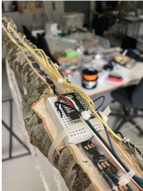
Figure 21 - The breakout board mounted on the branch, and LED strip underneath
