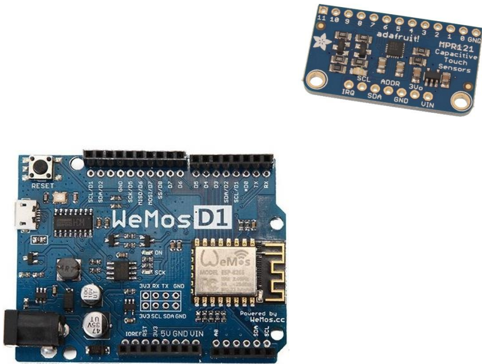
Figure 5 - Left: WeMos D1 R2 Wi-Fi board (Electrofun, 2023). Right: MPR121 Capacitive sensor breakout board (Electrokit, 2023)
