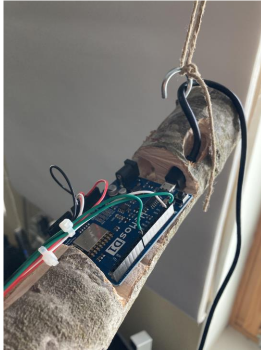
Figure 20 - The WeMos board mounted on the branch
