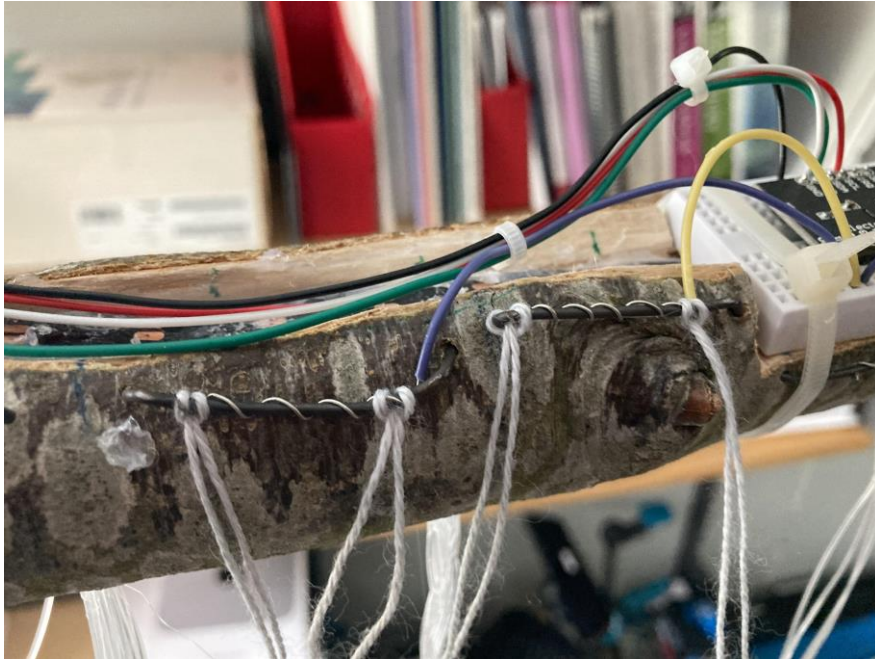
Figure 18 - The metal wires with twisted cables and and conductive threads
