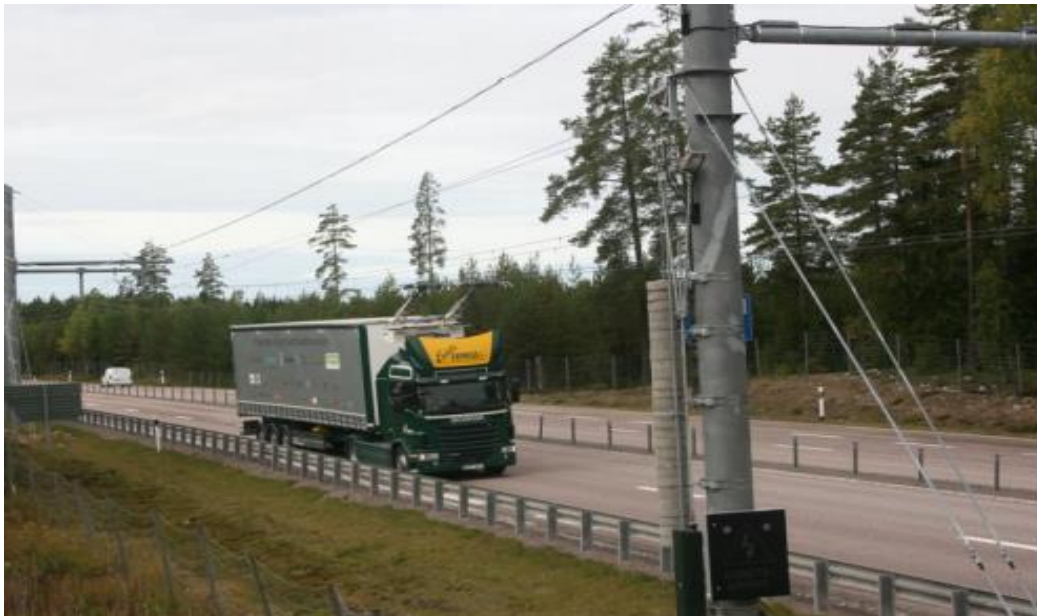
Figure 5: Conductive (catenary/overhead) ERS Concept (PIARC, 2018)
