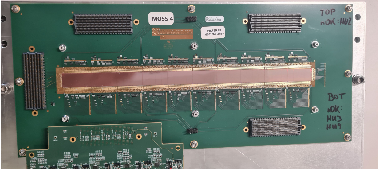
Figure 3.5: Picture by the author of a MOSS prototype connected to a printed circuit board, used for testing at the PS in September 2023. The MOSS is made up of ten units, divided into half-units, and each half-unit is made up of four matrices.
