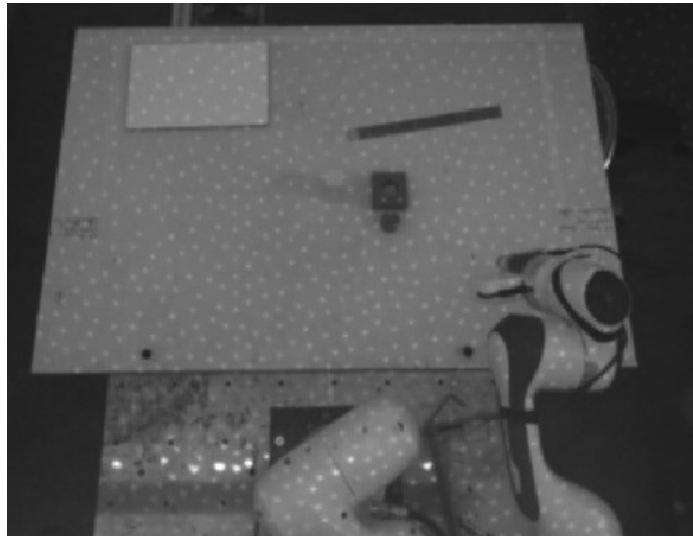
Figure 6.1: The figure shows the infrared speckle pattern with which depth data is collected by the top camera.
