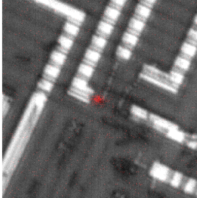
Figure 44: Light emission from a single InP NW detected by optical microscopy.
