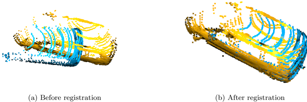
Figure 4: Point cloud registration of two LiDAR frames. Here the blue frame has been transformed to minimise its distance to the yellow cloud.
