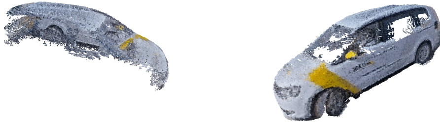
Figure 39: Point-NeRF rendering of half of a sequence of point cloud and video frames after 10 000 iterations.
