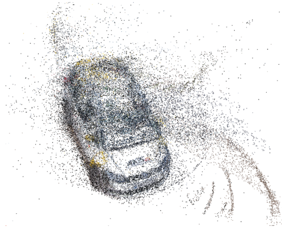
Figure 32: Point cloud produced by COLMAP using only the information from the image sequence and estimating camera poses via photogrammetry.
