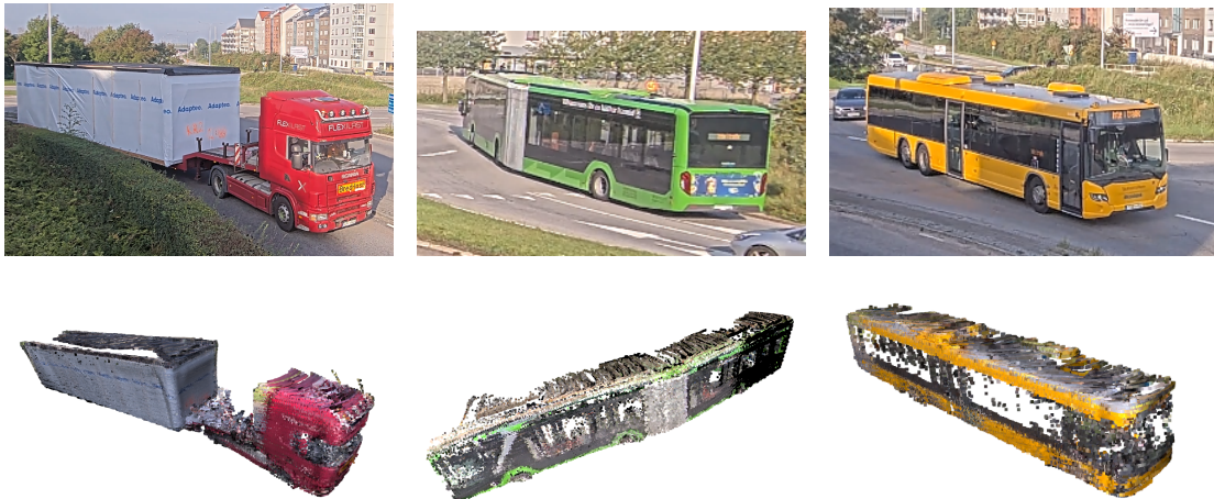
Figure 23: Point cloud aggregation with both initial frame alignment and ICP applied to other object in the roundabout scene with ground truth images for comparison.
