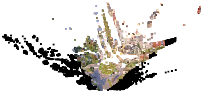
Figure 17: Illustration in the difference of Field of View for the LiDAR and the camera. The black points have been seen by the LiDAR but end up outside of the video frame after projection.
