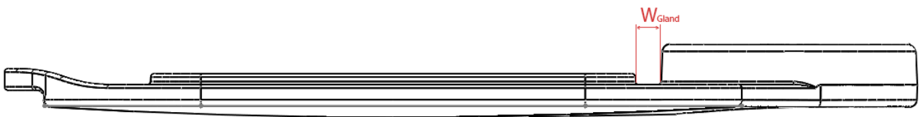
Figure 40: An illustration of the local gland and its smallest width W_{Gland}
