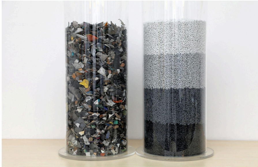
Figure 38: PC/ABS before & after recycle processing. Figure: mgg-recycling.com
