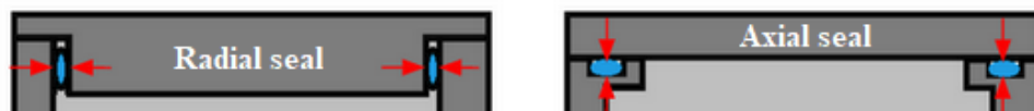
Figure 7: Illustration of the two gasket orientations, axial and radial. Figure: Siri Wetterstrand
