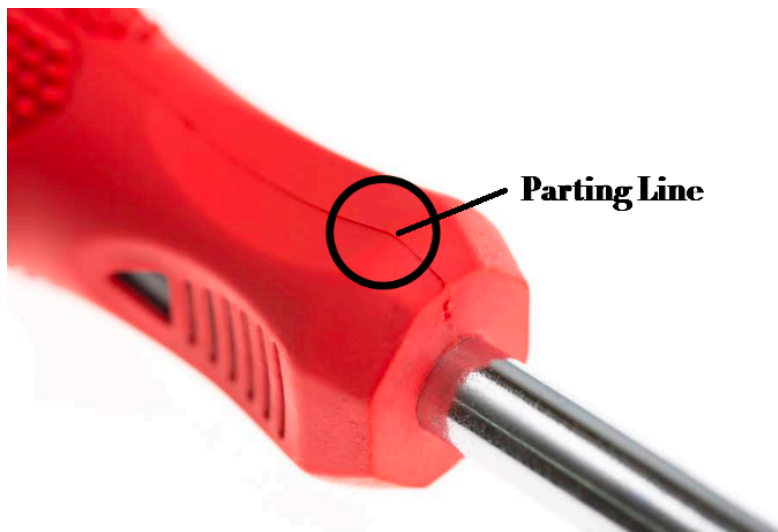
Figure 4: Shows a quality disturbance caused by the parting line.
