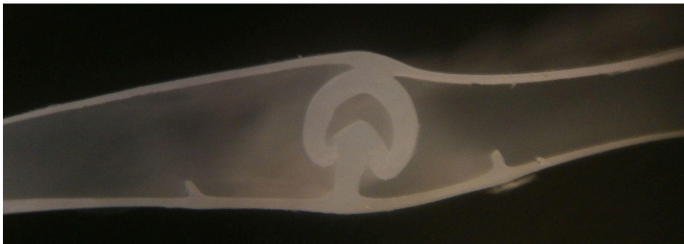
Figure 6: Even small details with high requirements of precision can be produced with extrusion.
