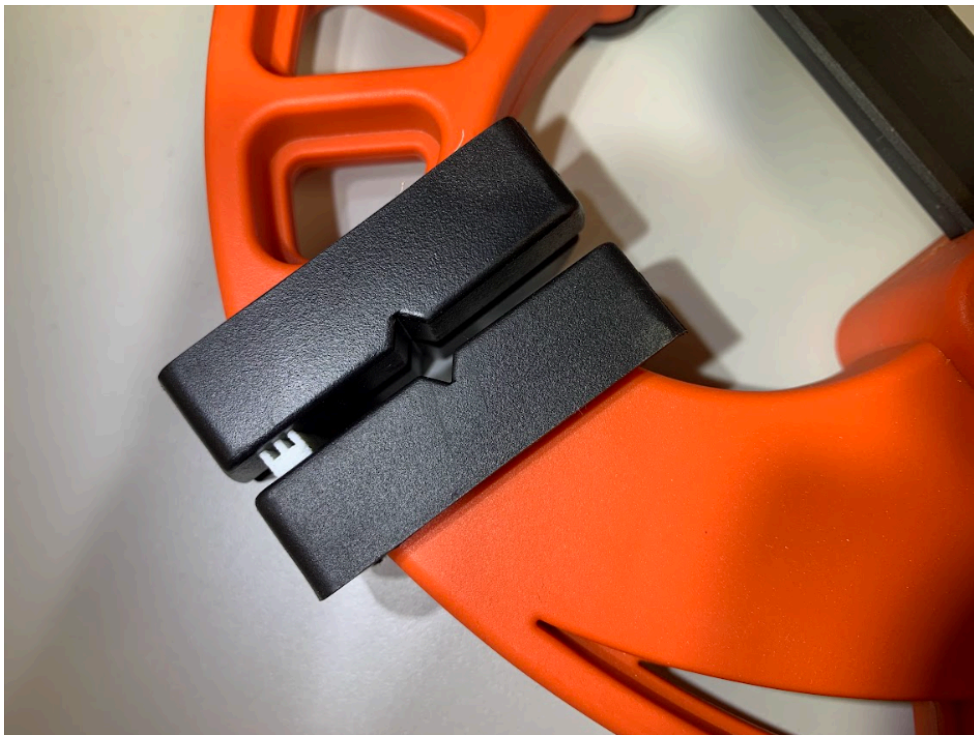
Figure 28: Set up with screw clamp under a microscope to study gasket deformation.
