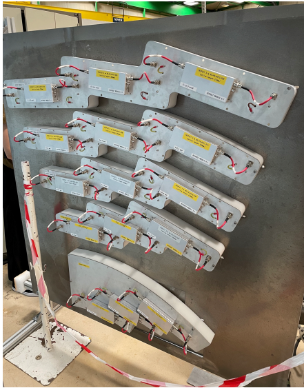
(c) Pre-amplifiers fixed on the back of the detector modules, mounted on the configuration holder.
