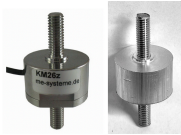
Figure 49: KM26z membrane-type force sensor in side-by-side comparison with the machined replica.
