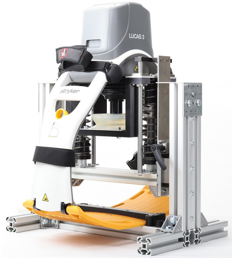
Figure 53: LISA III with the full LUCAS device mounted. The test equipment is tightly fit around, and is in the same range of dimensions as the LUCAS device.
