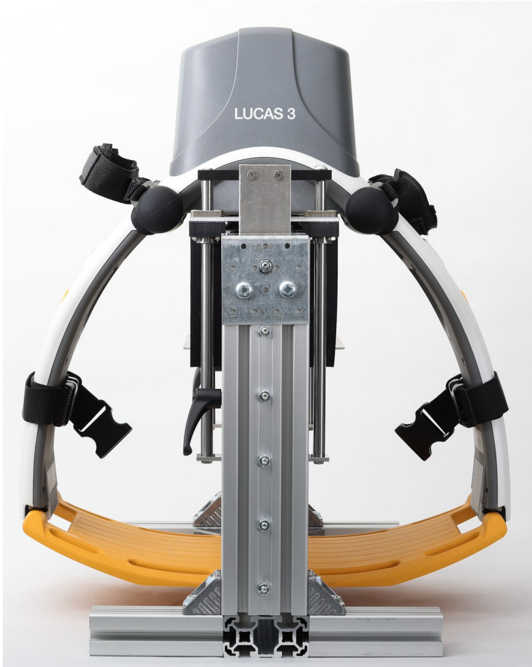
Figure 54: Side view of the LISA III test equipment with the full LUCAS device mounted. As can be seen in the figure, the equipment is within the dimensions for the LUCAS device, leading to desired minimal uptake of space.
