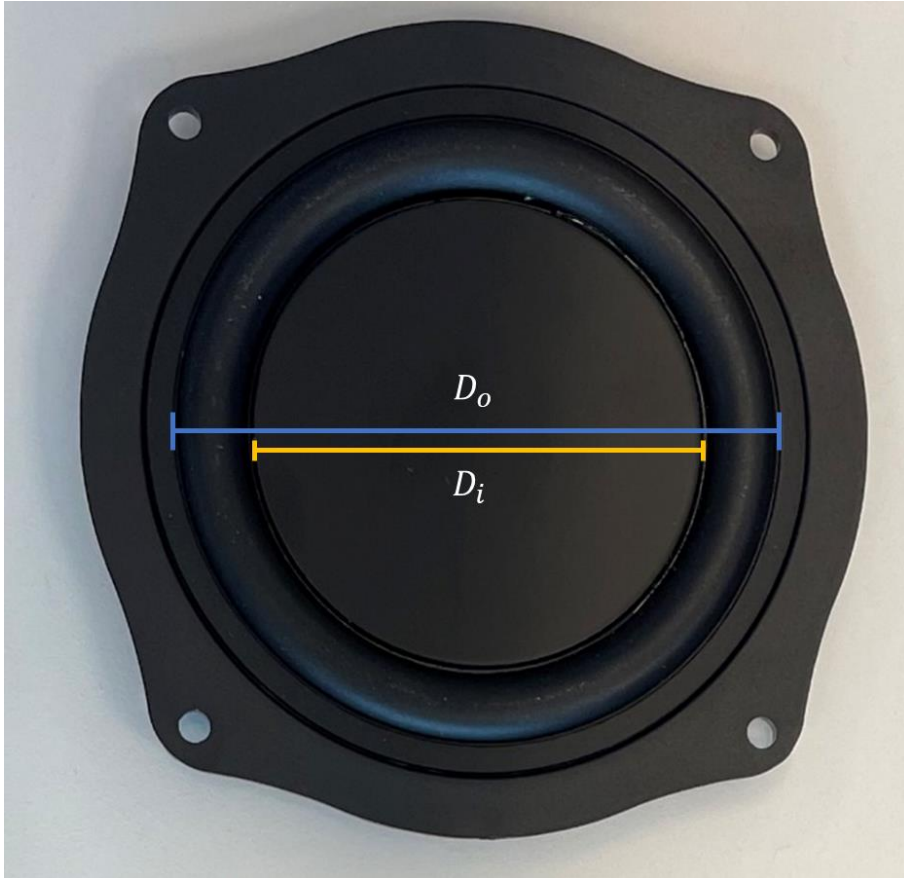
Figure 12: Measurements made on PR to calculate S_{dp}
