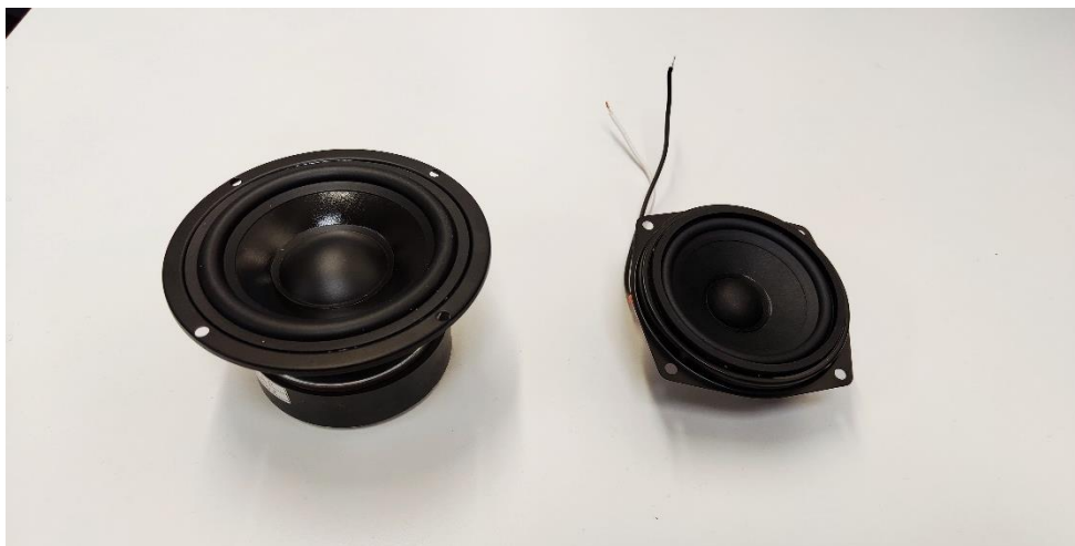
Figure 31: Selected speaker drivers, 4 and 3 inches respectively
