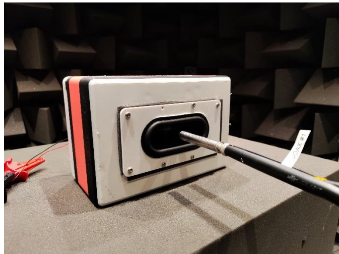
Figure 37: Near field measurement
