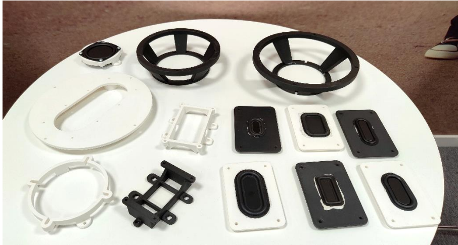
Figure 17: Some of the 3D printed PR mounts.
