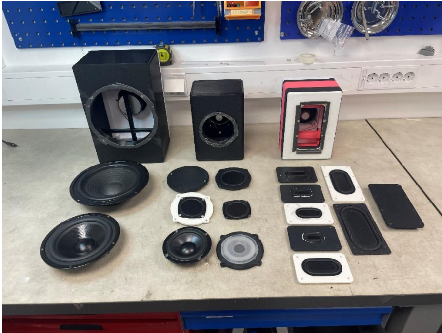
Figure 33: The three in-house made loudspeakers from the back, with the PRs that fit in their respective cavity.
