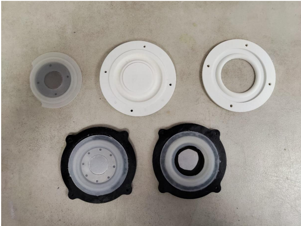
Figure 44: Self-made PR's consisting of silicone suspensions and steel-plates. The two white 3D printed parts are the moulds for creating the suspension.
