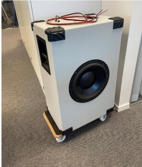
Figure 14: Frontside of the modular subwoofer
