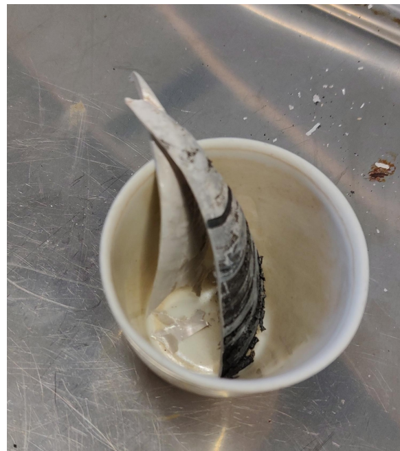
Figure 3.6: A shell from the initial testing, showing the separation of layers. Heated from about 400 °C to 500 °C, taking approximately 12 minutes.
