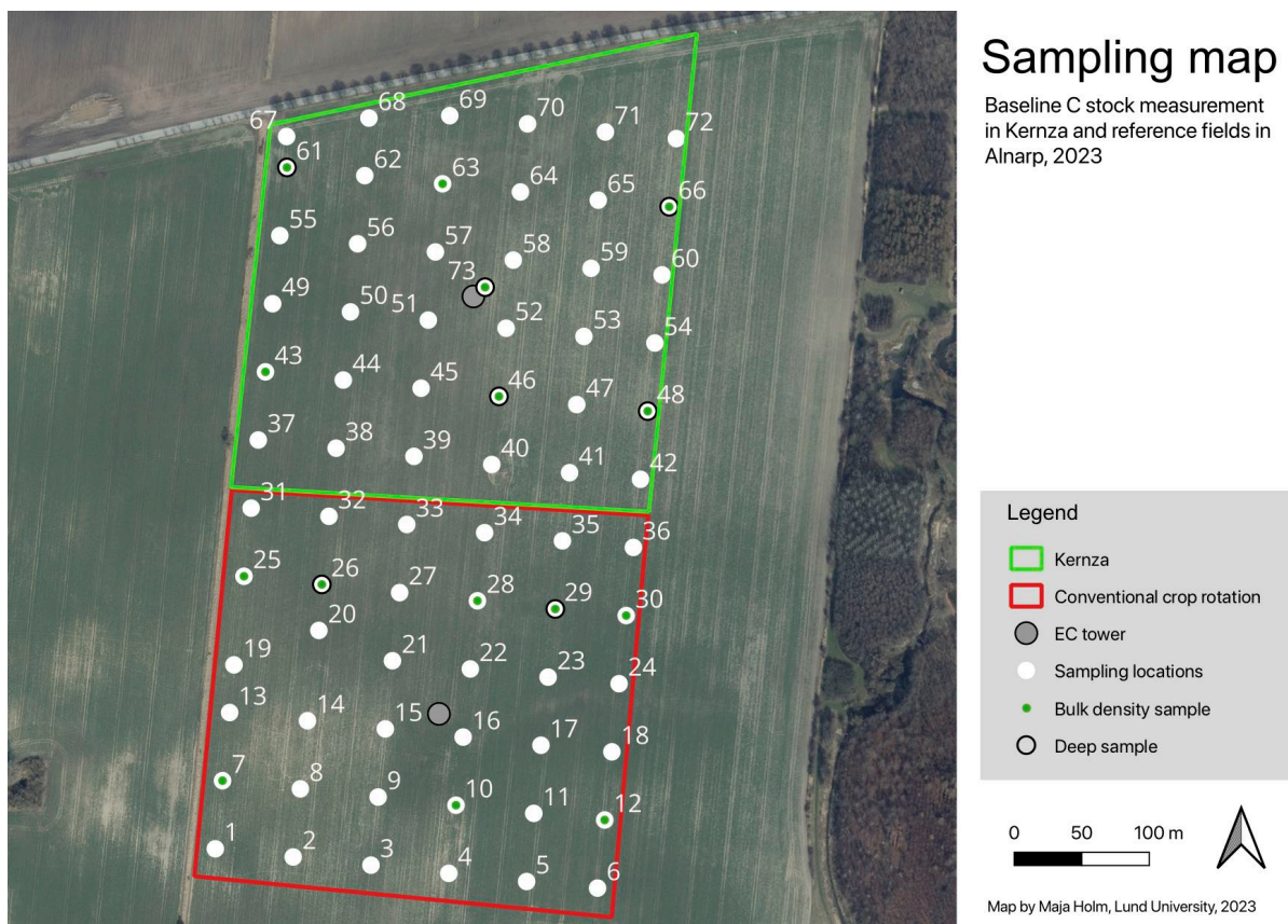
Figure 1. Map of all 73 sampling locations, both SOC and BD, at the Alnarp research site. EC towers and deep samples are also included.
