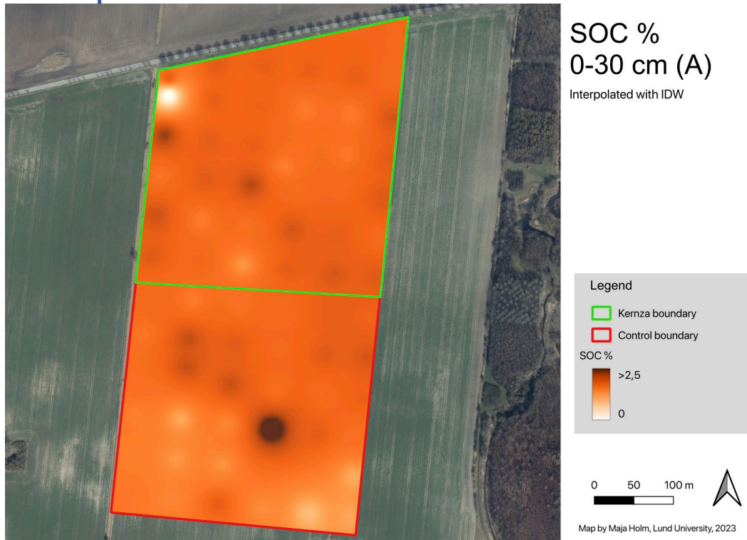
Figure 11. Soil organic carbon (SOC) content of the Kerna™ and control plots at 0–30 cm, interpolated across the total area. Based on 73 field samples collected at the research site in 2023. The resolution was 0.1 m.
