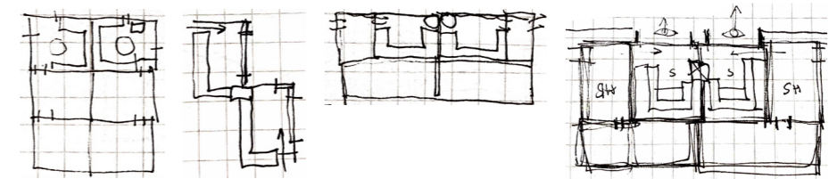
The sauna was studied through its connection to the outside view. The movement inside the building was also studied. The flows between showers, saunas and outside swimming had to be natural.
