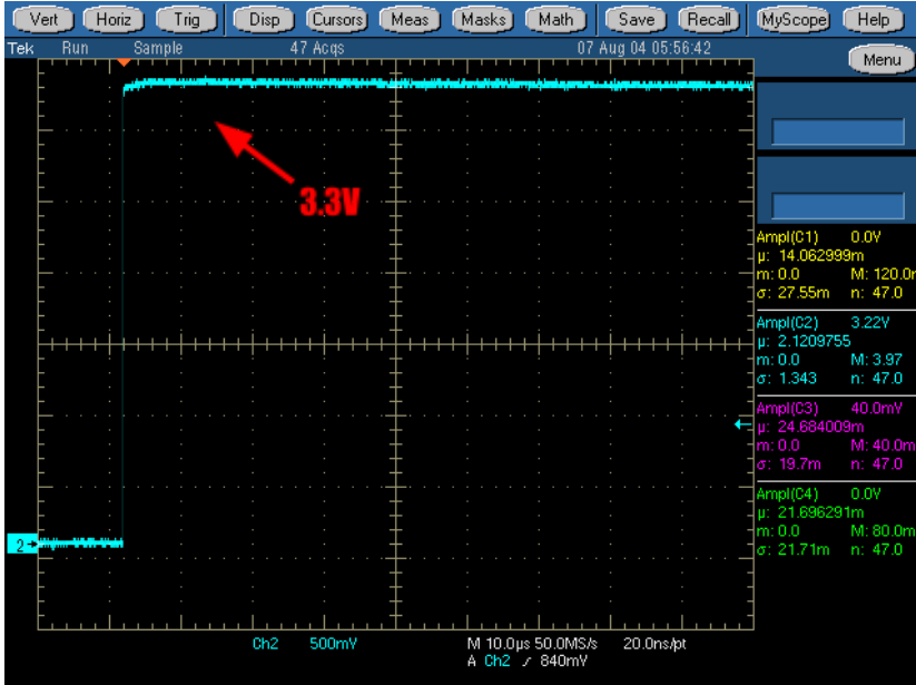
Figure 4.24: VDD measurements on the LED resistors.
