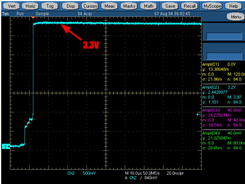
Figure 4.27: VDD measurements after the PU resistor on connector 1.
