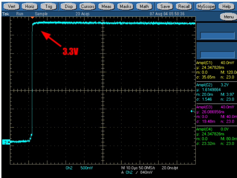
Figure 4.22: Measurements on the main VBAT power node.
