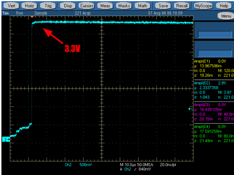
Figure 4.29: VDD measurements after the PU resistor on the button.
