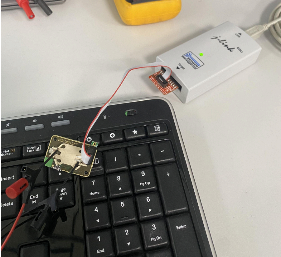
Figure 3.18: Flashing the PCB using J-Link.
