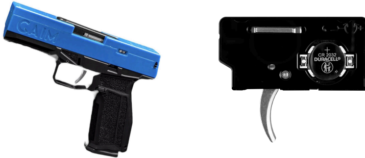
Figure 1.1: GAIM product, dummy gun and the trigger unit [1].
