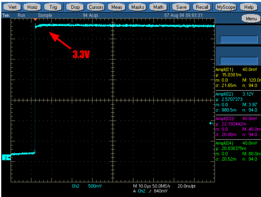
Figure 4.28: VDD measurements after the PU resistor on connector 2.
