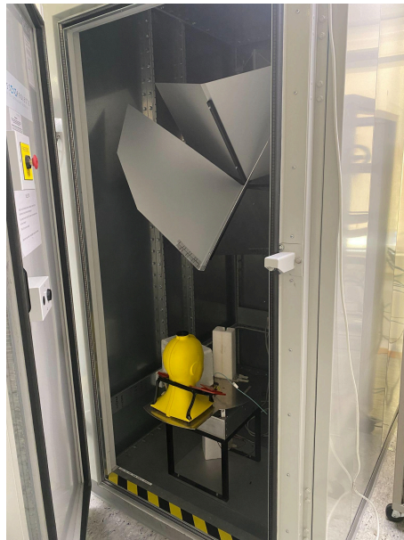
Figure 3.19: RF chamber for radiated measurements.
