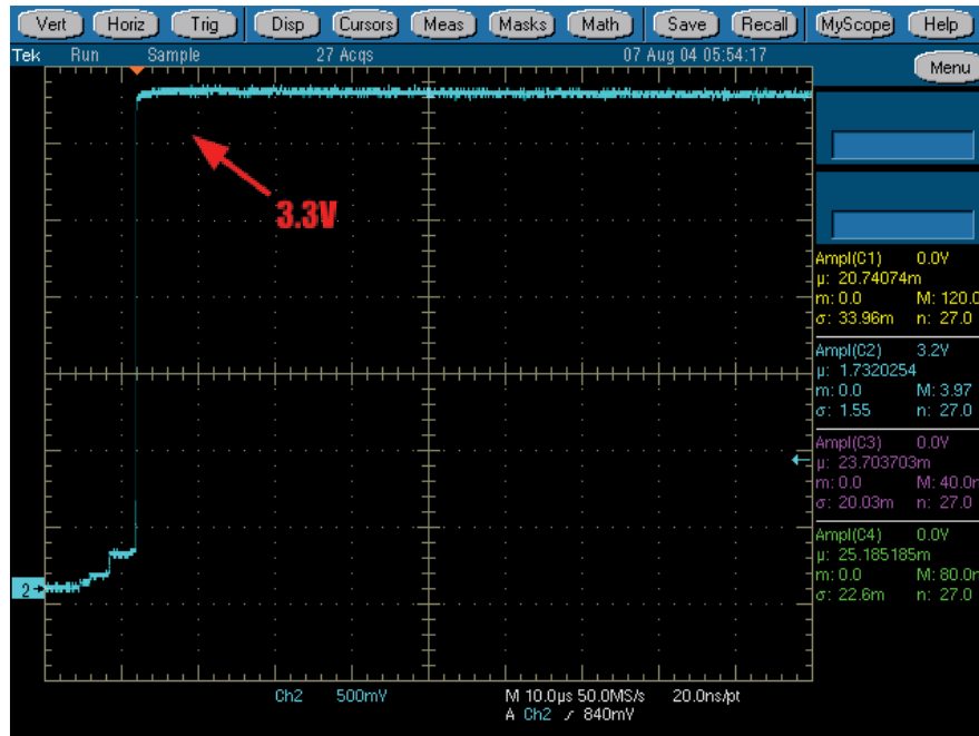
Figure 4.23: Measurements on the first (and only) VBAT power plane.
