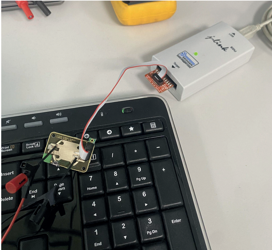
Figure 3.18: Flashing the PCB using J-Link.
