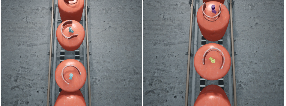
Figure 3.10 Images from the Random Cap and No-Cap material dataset which displays randomized material of Caps and No-Caps.
