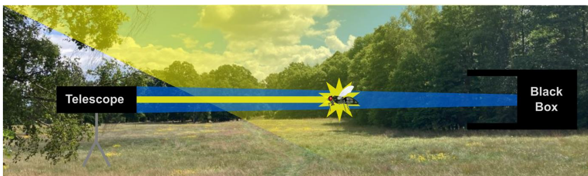
Figure 1: Schematic of experimental setup used to catch sunlight reflected by free flying insects.
