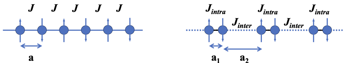
Figure 2.4: Geometry of a uniform 1D Heisenberg chain (left) and an alternating 1D Heisenberg chain (right).
