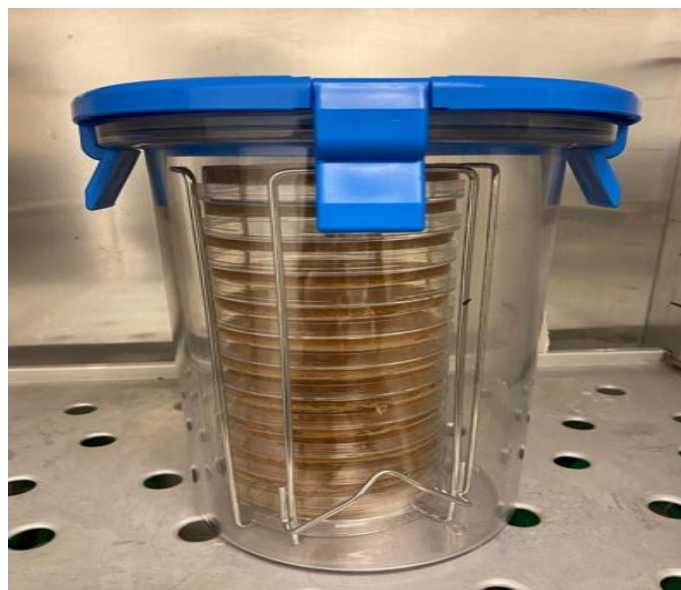
Figure 10) agar plates are placed in air tight container for incubation
