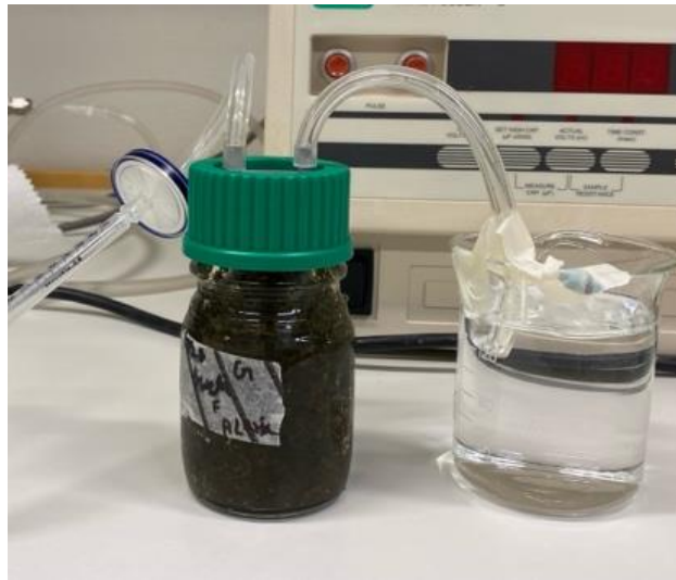
Figure 8 Fermenter and anaerobic condition set up .
