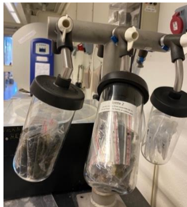
Figure 14 freeze-drying seaweed sample using Labconco Freeze Dry System Lyph-lock 12.
