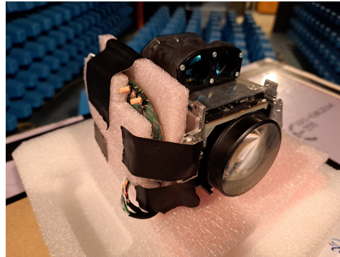
Figure 3.7: The PCBs and camera block are placed similarly to their placement inside the whole camera with the help of plastic foam and tape.
