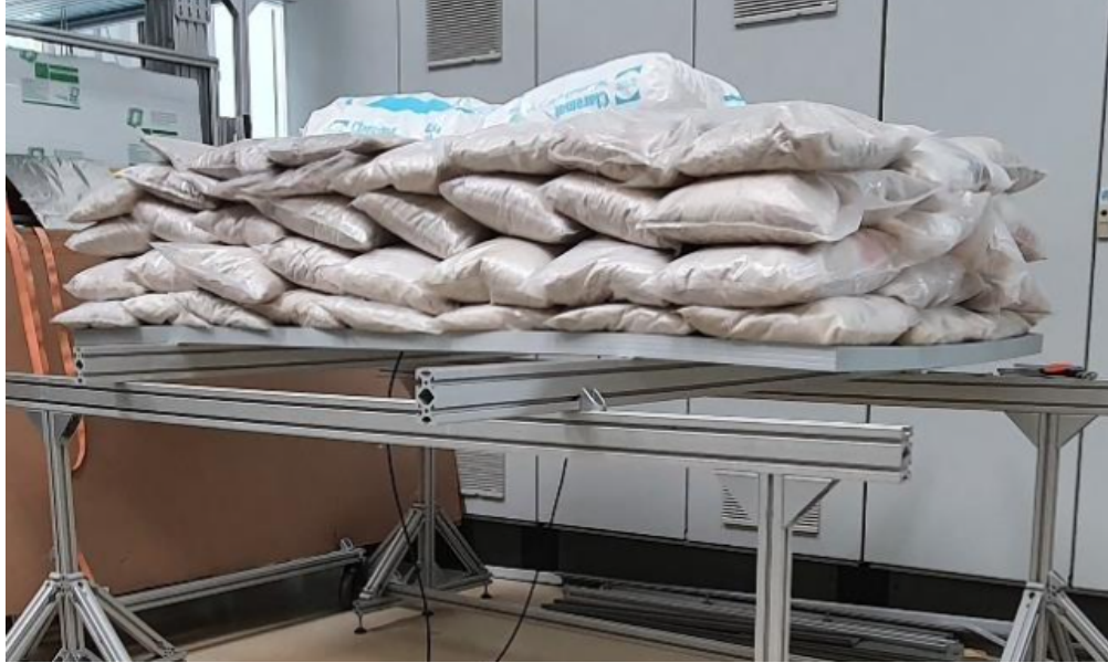
Figure 18: Mechanical load test of 5800 Pa, can be made both in this way with weighted bags or with a machine that applies the pressure. Picture from RWE.
