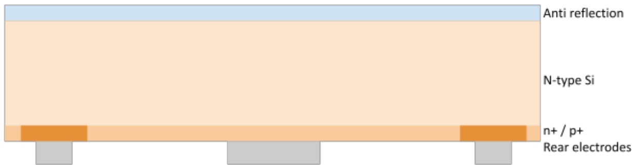
Figure 8: Schematic structure of a basic IBC solar cell
