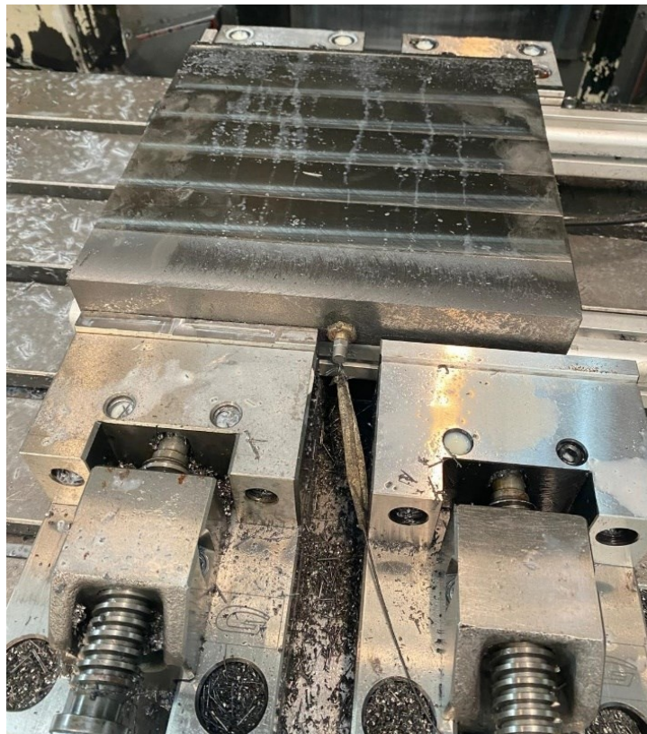
Fig 30. Clamping setup used during this thesis. Coolant leftover from a intermediate clean-cut can be seen on the workpiece.
