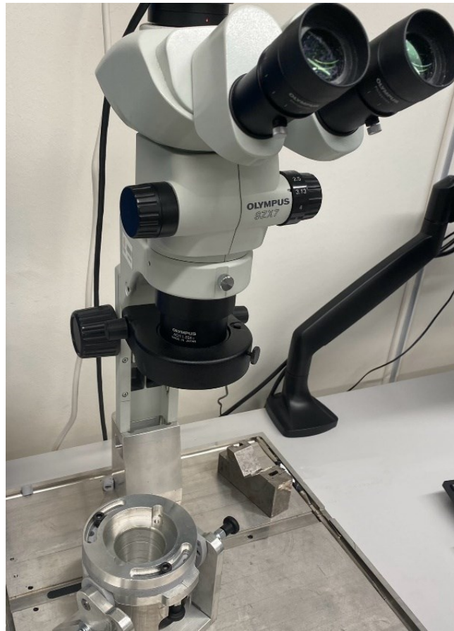
Fig 31. Olympus SZX7 optical microscope used in this research, with adjustable toolholder visible.
