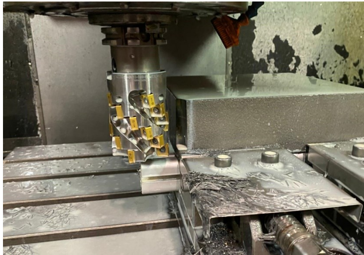
Fig 27. Image of an interrupted pre-machining process, of a workpiece equivalent to the ones used in this research.
