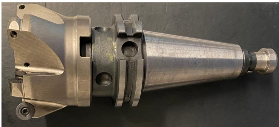
Fig 19. Image of combined tool and tool holder with a single insert attached.
