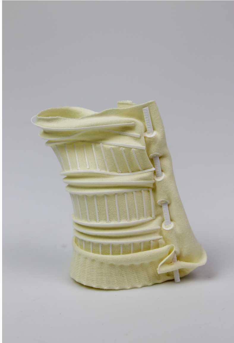
Fig. 7.7.8 Early iterations of the tower prototypes, in neutral and compressed states, showcasing the geometry's effect on structural integrity
