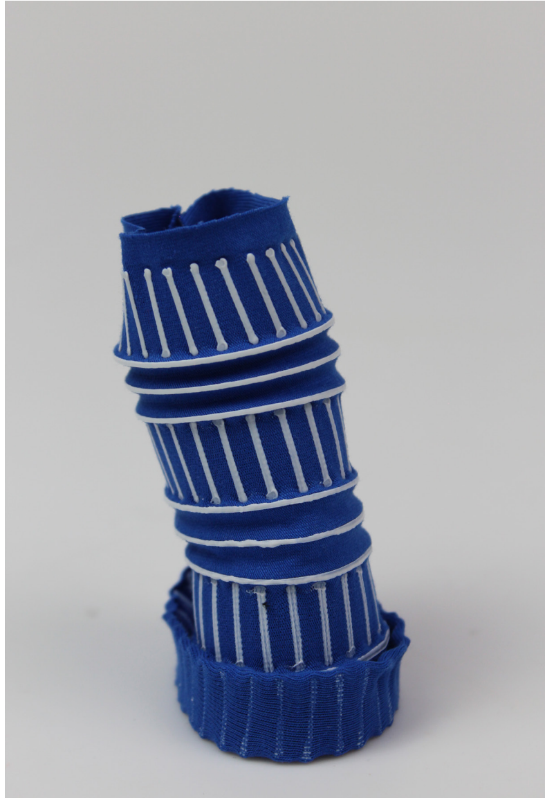
Fig. 7.7.9 Early iterations of the tower prototypes, in neutral and compressed states, showcasing the geometry's effect on structural integrity
