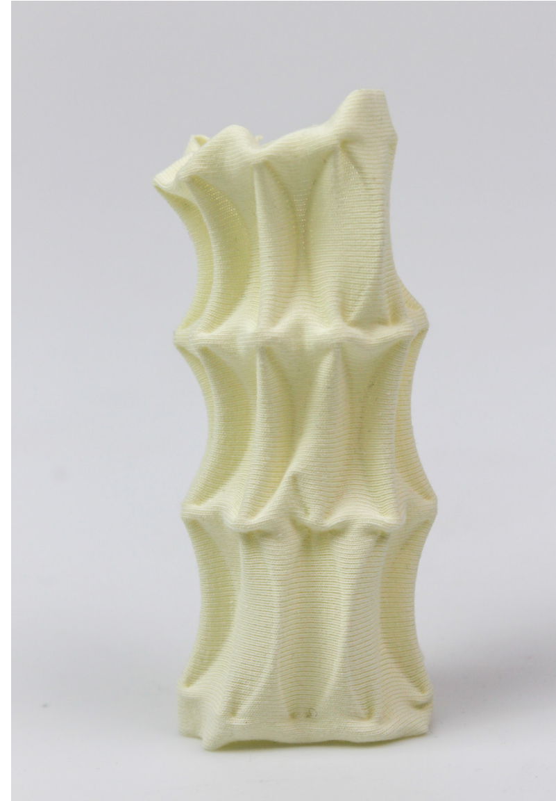
Fig. 7.3.12 PLA parentheses textural tower Material Behavior: Arching
