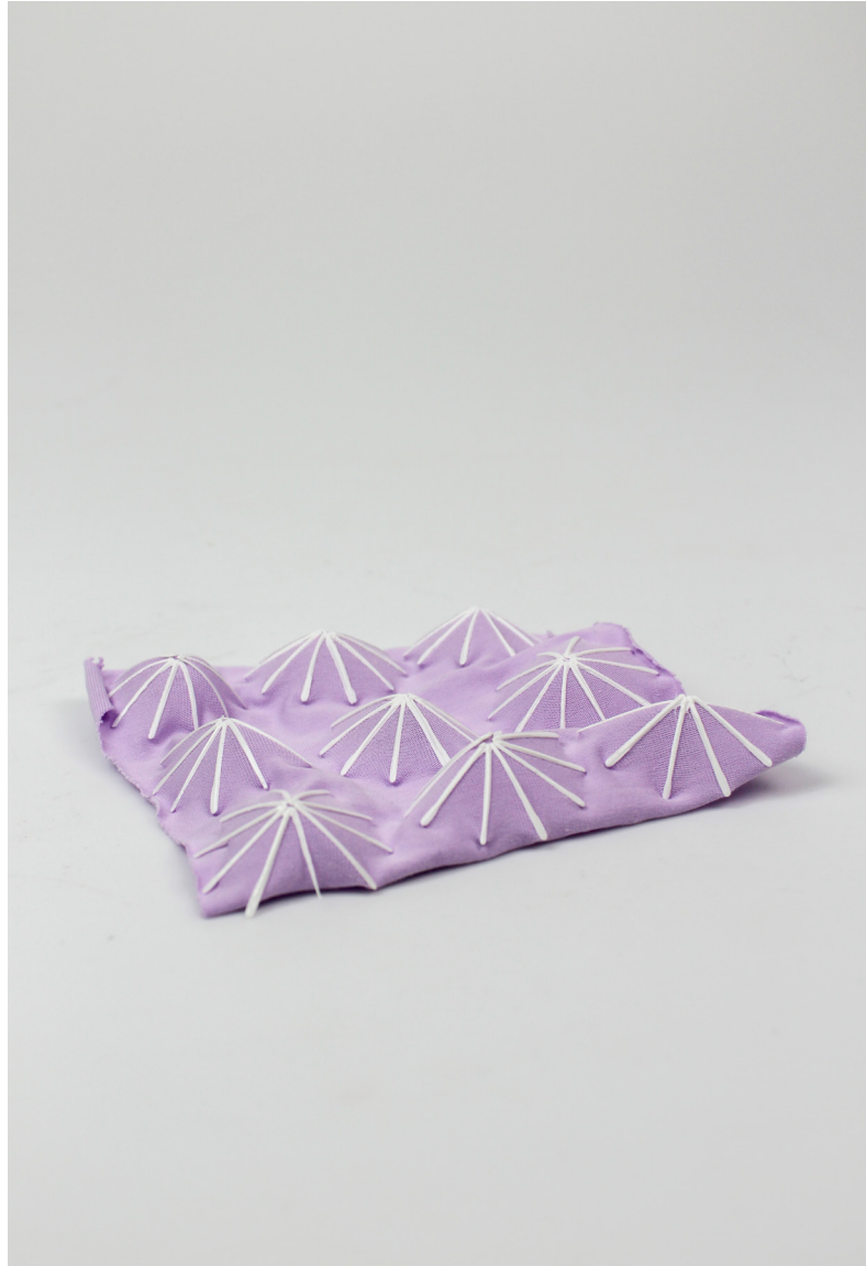
Fig. 7.3.21-22 Cotton and PLA, structural warping Material Behavior: Peaking
