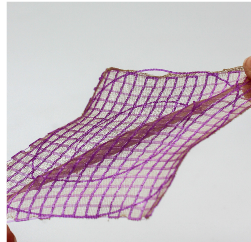
Fig. 9.6 Nylon reinforced with a TPU grid and spiral
