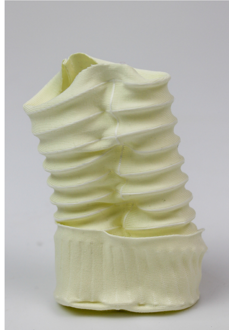
Fig. 7.3.16 Ribcage rolled base experimental tower Material Behavior: Wrinkling + Bending
