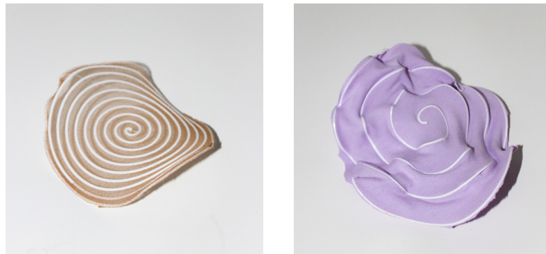
Fig. 7.6.4-5 Identical PLA geometries printed on Nylon and Cotton, displaying different warping behaviors Material Behavior: Arching vs Puckering + Wrinkling
