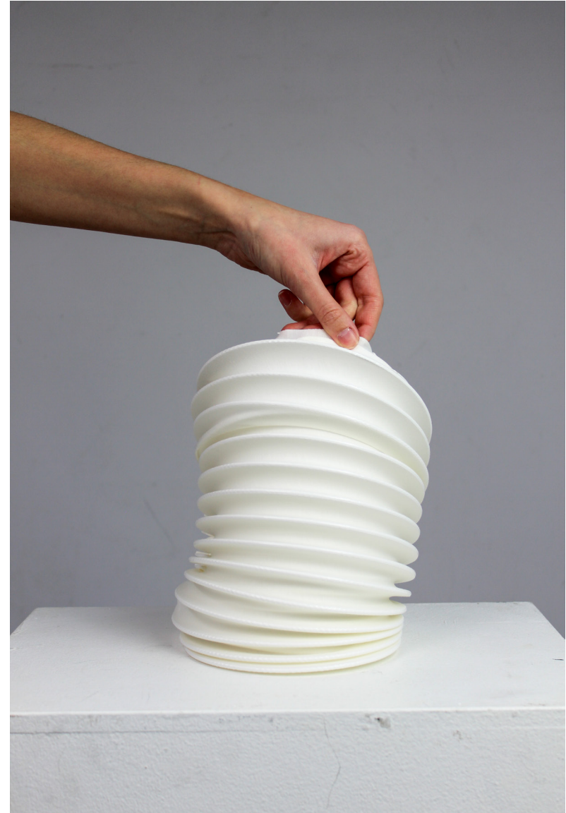
Fig. 8.3.7-8 Folded single column configuration of the dynamic structure, compressed and expanded
