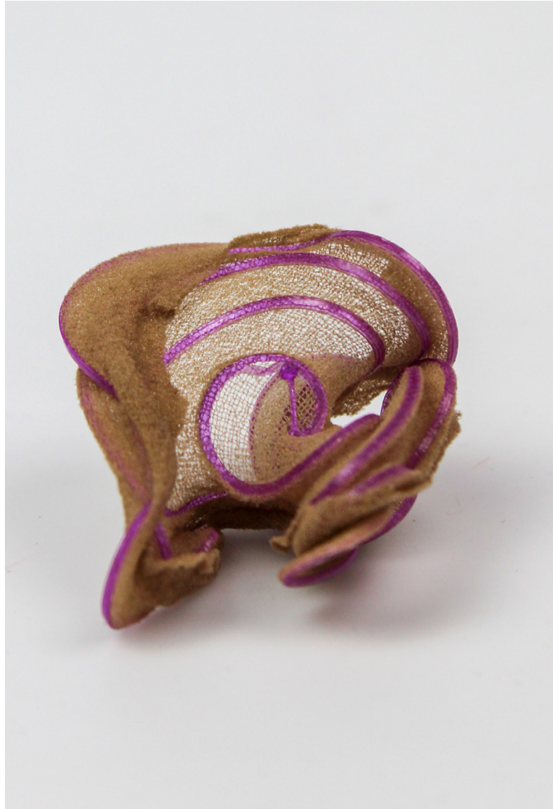
Fig. 7.3.27-28 Nylon and TPU, structural warping Material Behavior: Curling + Puckering + Wrinkling
