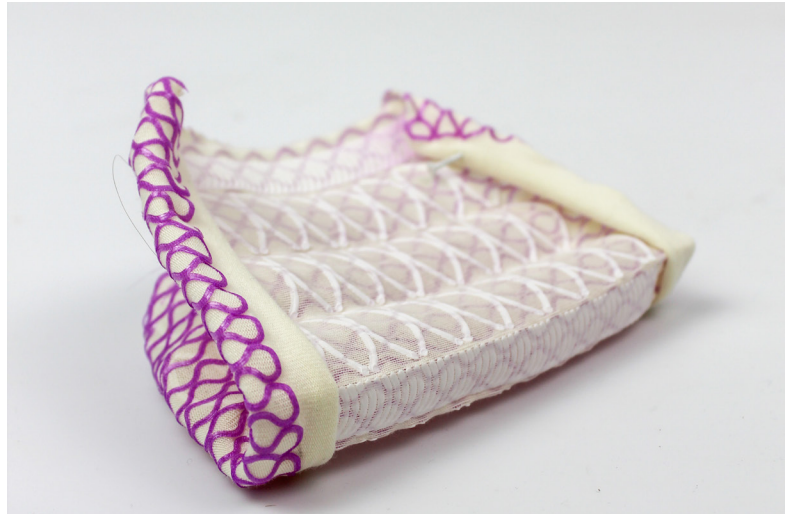
Fig. 9.5 Multi-material printing on separate fabric sides
