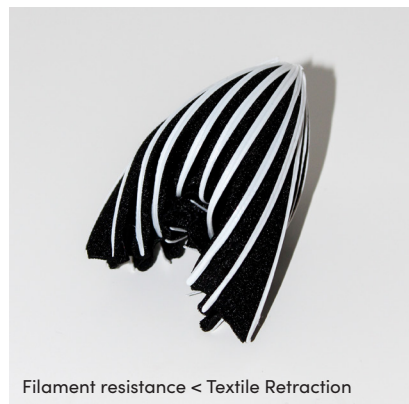
Fig. 7.6.2 Diagrams depicting the balance between the forces of filament resistance and textile retraction in Test Geometry 2
