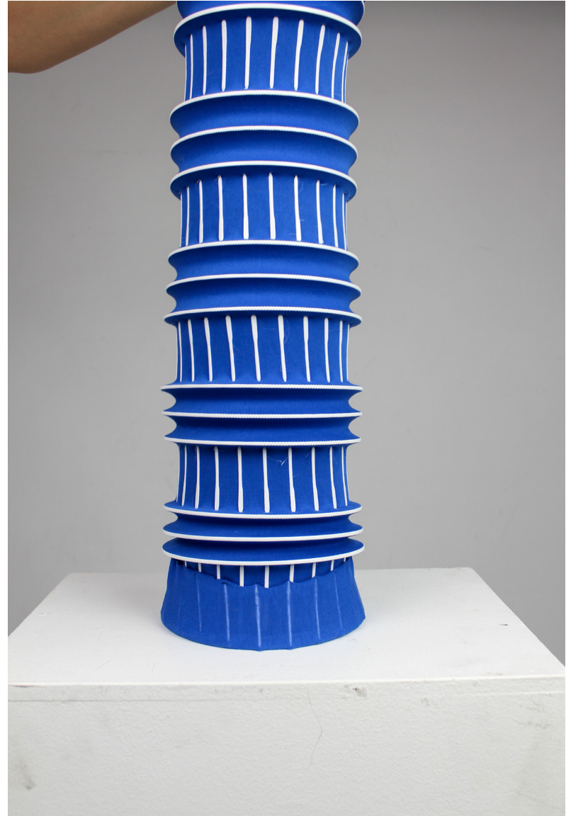
Fig. 8.2.9-10 Tower prototype in rest (compressed) vs expanded
