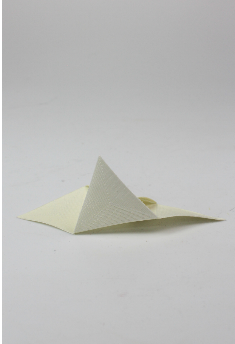
Fig. 7.3.19-20 Cotton and PLA, structural warping Material Behavior: Folding
