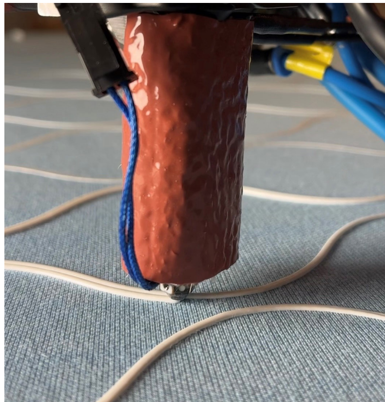
Fig. 7.4.3 Hemera extruder with a nozzle height too high
