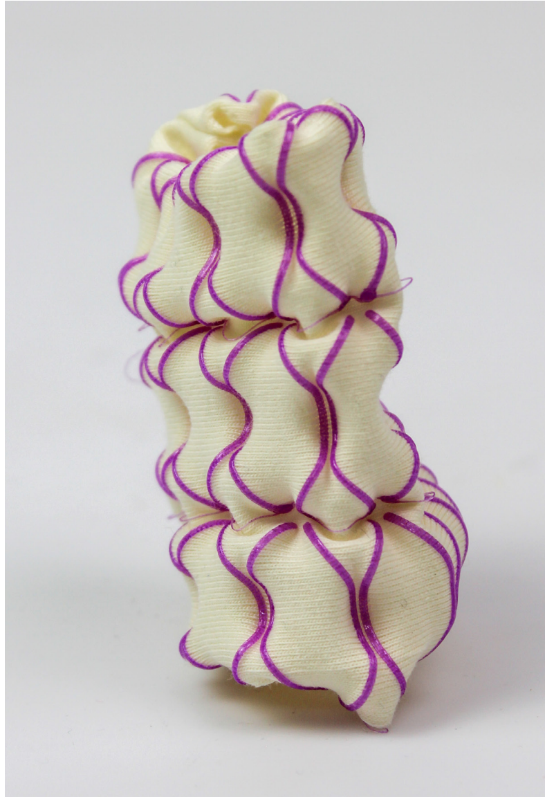
Fig. 7.3.11 TPU parentheses textural tower Material Behavior: Wrinkling + Arching + Puckering
