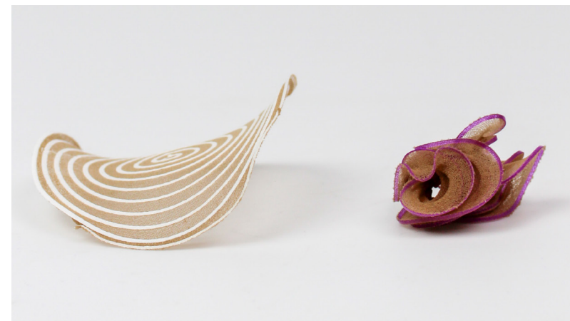
Fig. 7.5.1 PLA/Cotton structural warping Material Behavior: Puckering + Arching
