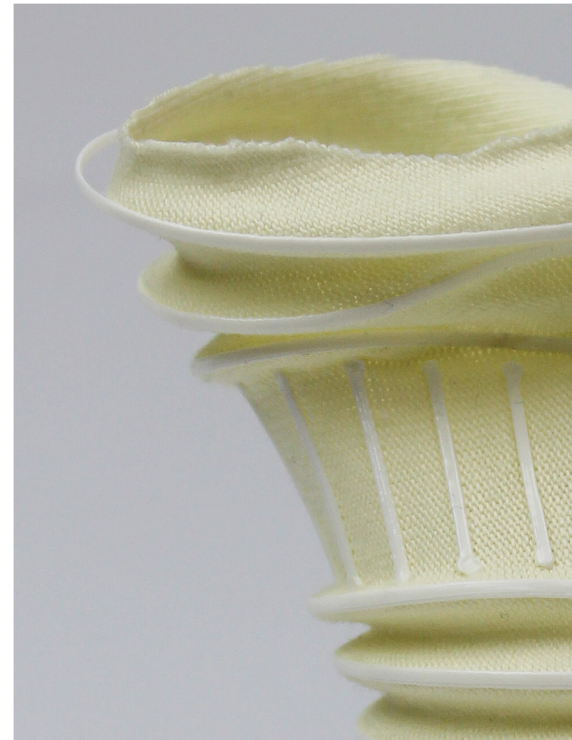
Fig. 7.4.1 PLA/Lycra, adhesion lost due to too high of a nozzle height during print
