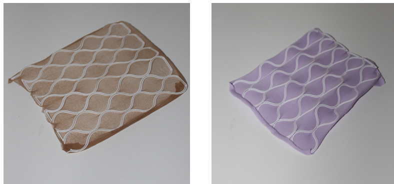
Fig. 7.6.6-7 Identical PLA geometries printed on Nylon and Cotton, displaying different warping behaviors Material Behavior: Folding vs Folding + Arching
