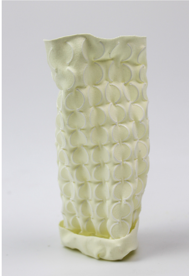
Fig. 7.3.13 Half-circle textural tower with rolled base Material Behavior: Puckering
