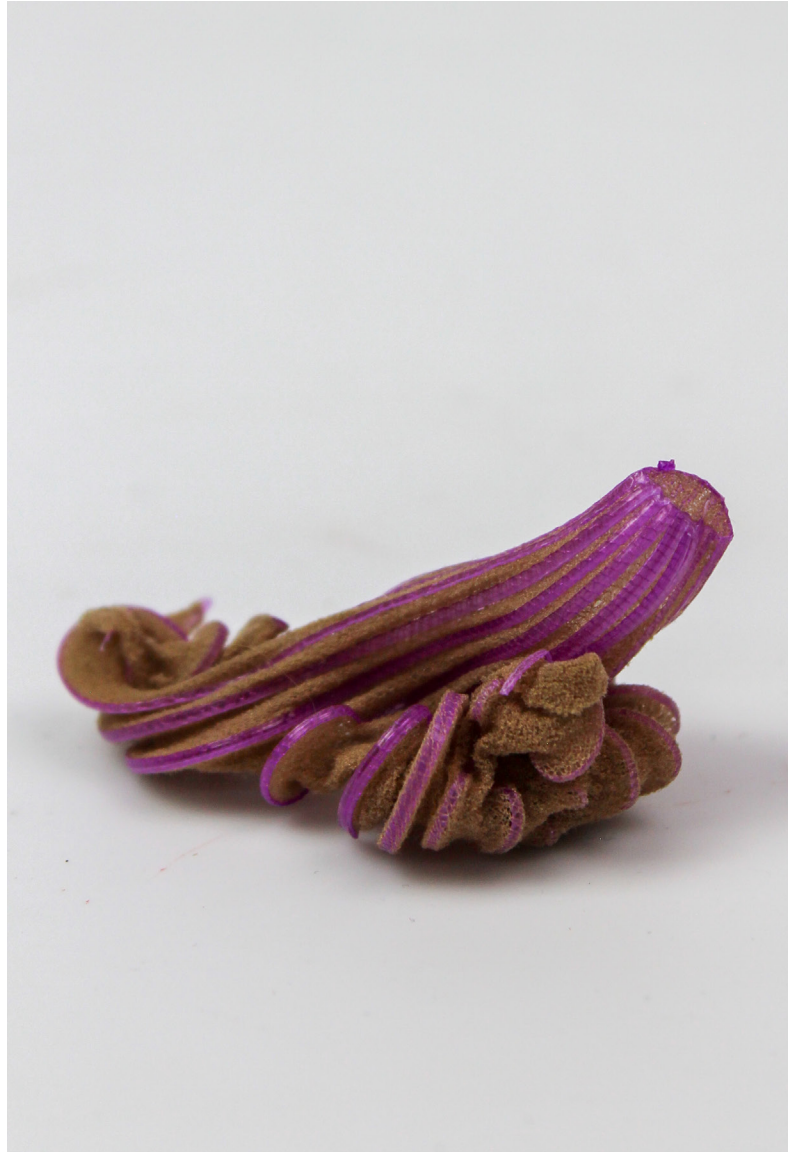
Fig. 7.3.23-24 Nylon and TPU, structural warping Material Behavior: Curling + Puckering + Wrinkling
