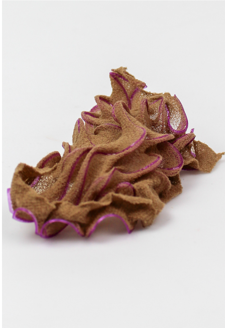
Fig. 7.3.25-26 Nylon and TPU, structural warping Material Behavior: Puckering + Wrinkling
