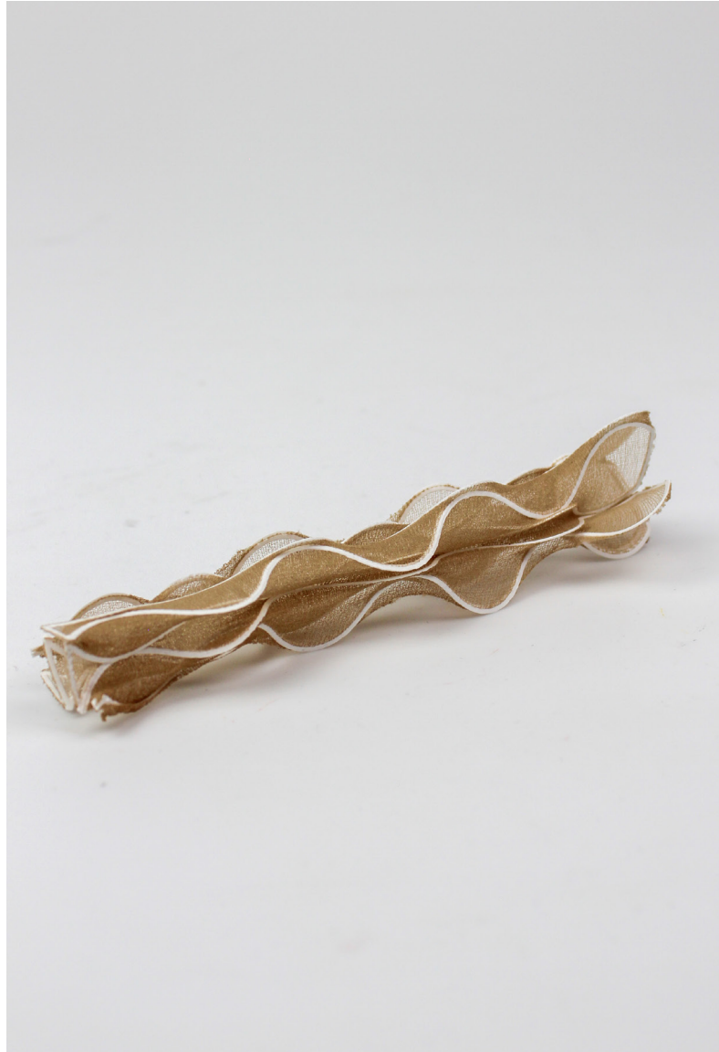
Fig. 7.3.17-18 Nylon and PLA, structural warping Material Behavior: Folding
