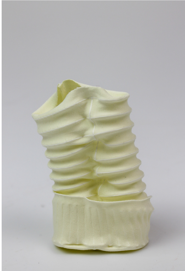
Fig. 7.7.6 Early iterations of the tower prototypes, in neutral and compressed states, showcasing the geometry's effect on structural integrity
