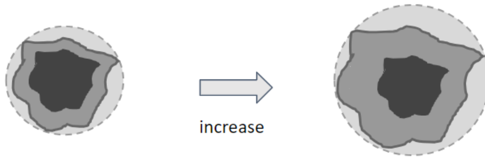
Figure 2.5. Outwards growth of biofilm on the surfaces of Cella support material leading to an increase in cross-section of biofilm surface for contact to wastewater (dashed line), when biofilm (dark gray area) is increasing in thickness, while thickness of the boundary layer (light gray area) stays the same.
