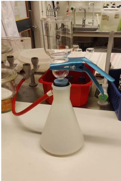
Figure 4.6. Experimental setup of vacuum flask used to filtrate water sample through a micro-glass fibre filter to measure TSS.
