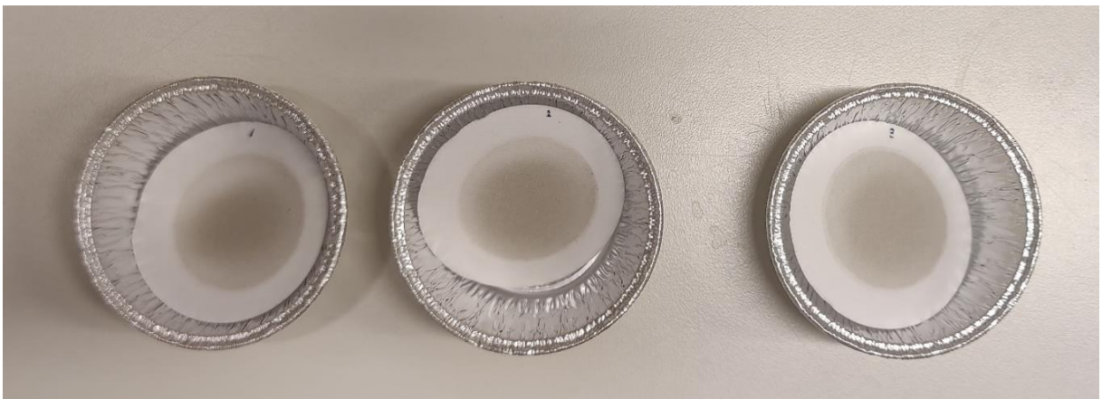
Figure 5.3. The micro-glass fibre filters after TSS-analysis of raw rainwater. The dark circles are the residues from the raw rainwater.
