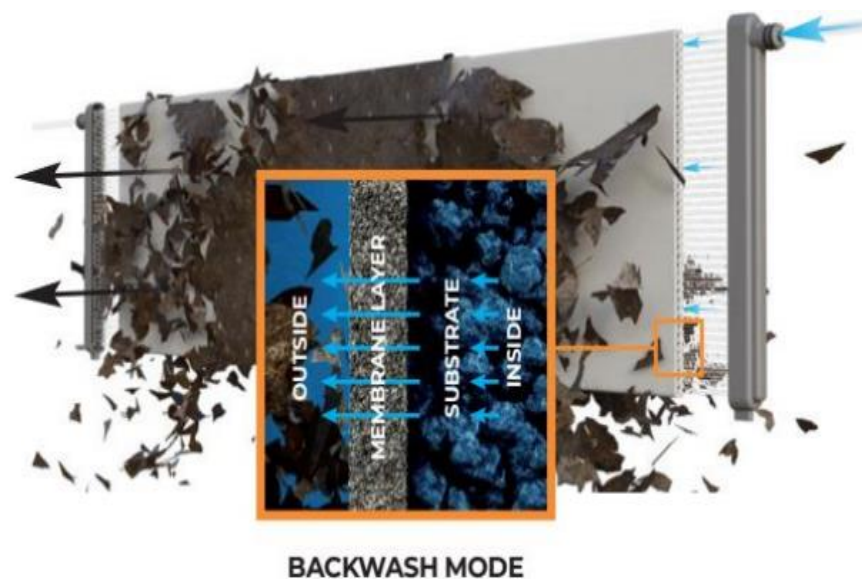
Figure 3.2. Illustration backwash mode (Cembrane A/S, n.d-b). Picture retrieved with consent from Cembrane A/S.
