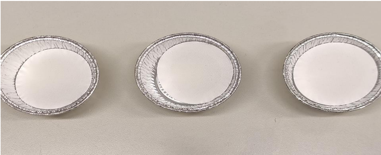
Figure 5.4. The micro-glass fibre filters after TSS-analysis of the permeate.
