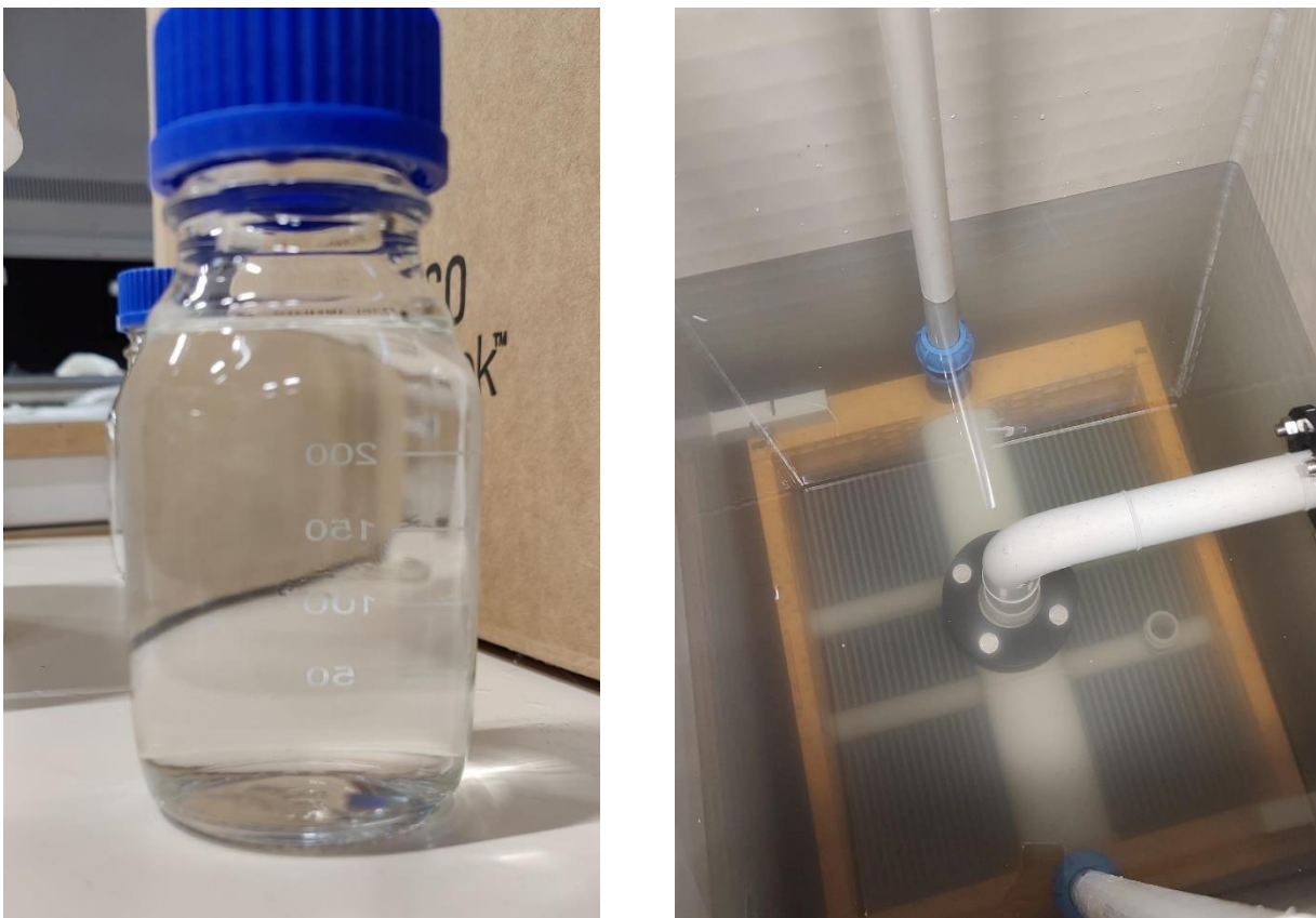
Figure 5.1. Raw rainwater sample from Kemicentrum rooftop to the left. Rainwater in the membrane tank with visible cloudiness to the right.
