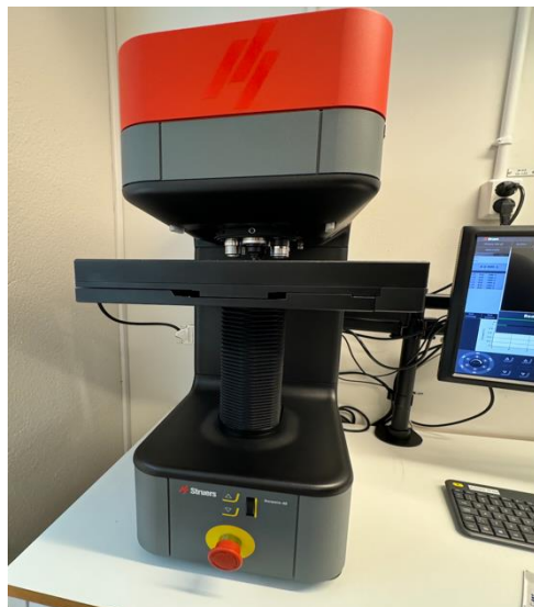
Figure 14: Hardness test machine Struers Duramin 40 AC used in the experiments.
