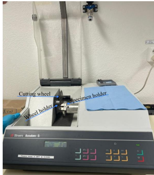
Figure 10: Cutting machine Struers Accutom-5 used in the experiments.
