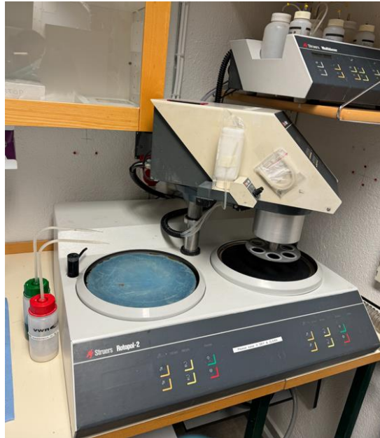
Figure 13: Photograph of a semi-automated grinding/Polishing machine Struers Rotopol-2 used in the experiments.
