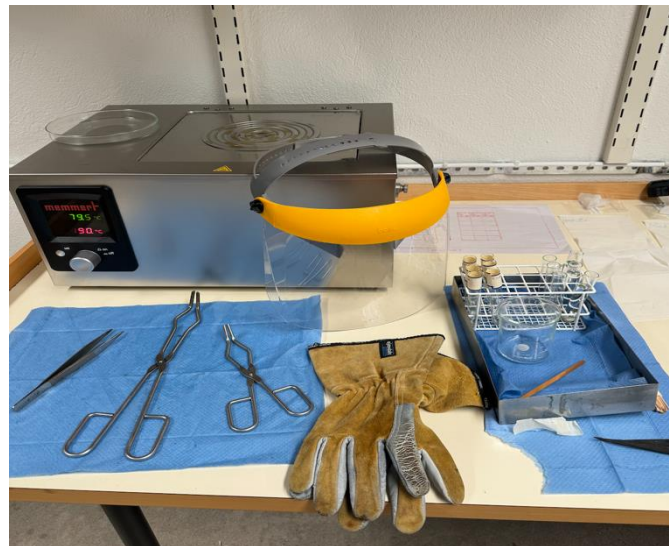
Figure 9 : Oil bath One-7 by Memmert and personal protective equipment used in the experiments.
