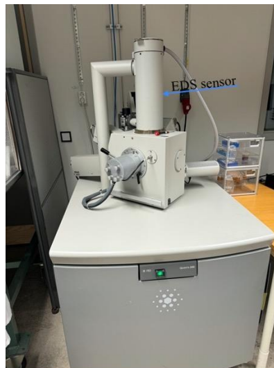
Figure 16: SEM FEI Quanta 200 MKII instrument used in this work
