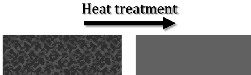
Figure 4: As casted with solid precipitates (left). Homogenized composition (right) (Viklund,2019).
