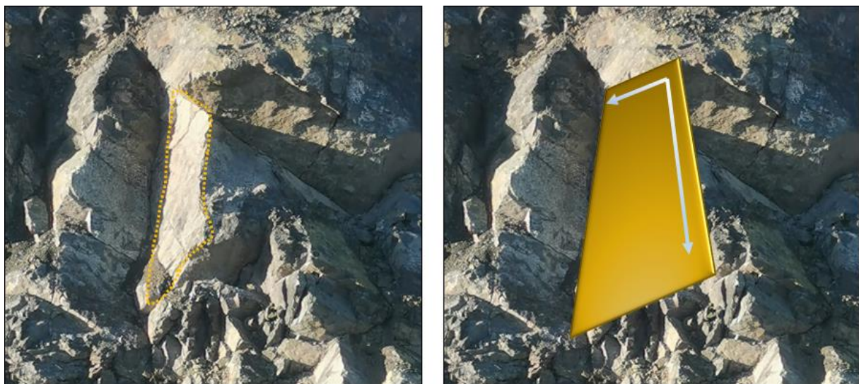
Figure 23. Schematic illustration showing a polygon fitted to the orientation of an exposed fault plane. The method allowed for strike and dip data to be acquired without interference from the magnetic properties of the mineralisation.
