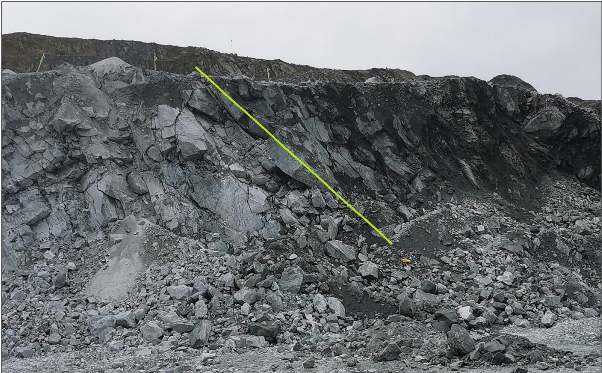
Figure 9. Transitional contact between the foot wall dolomite (left) and skarn alteration (right), Tapuli Central pit.
