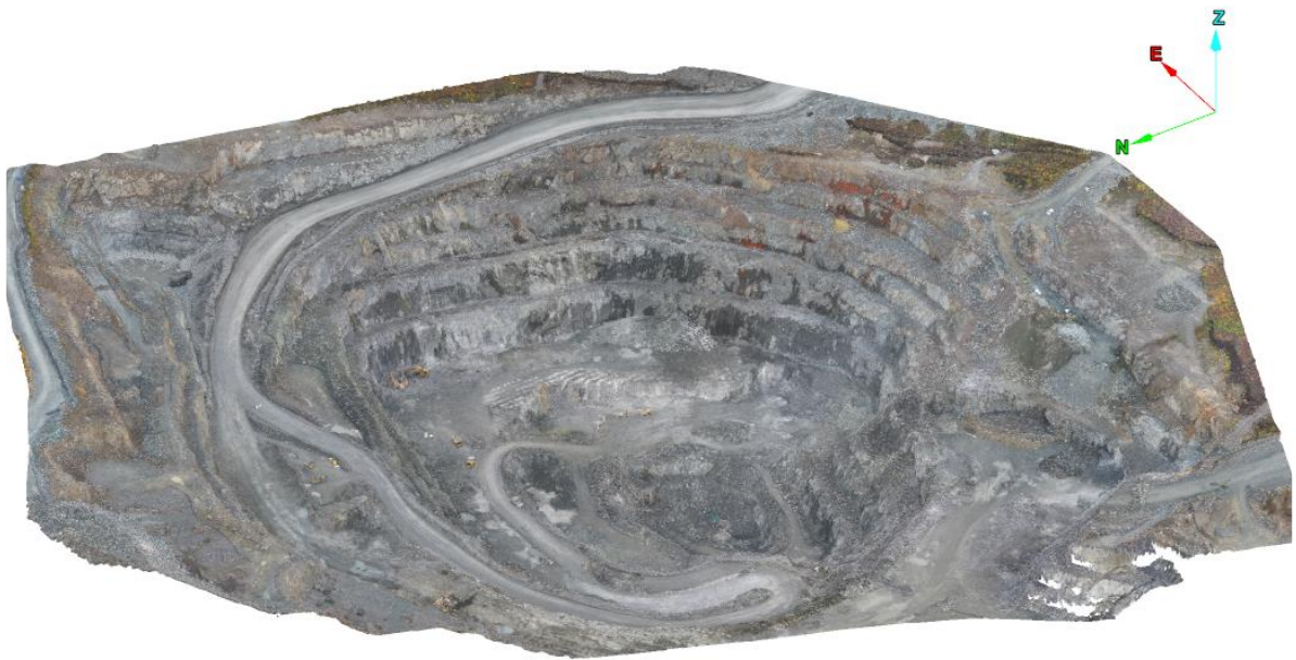
Figure 22. 3D model of Tapuli Central pit generated from drone photography and surface reconstruction. The diameter of the pit is roughly 500 m.
