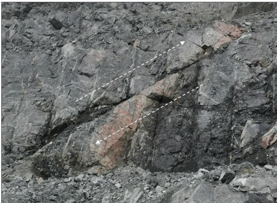
Figure 17. Moderately dipping reverse fault with a displacement of approximately 5 m in the North pit hanging wall.
