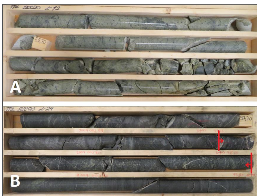
Figure 11. The three major types of skarn alterations in the Tapuli deposit: Clinopyroxene-tremolite skarn (A), magnetite-actinolite skarn (B outside red markers) and serpentinite skarn (B inside red markers).
