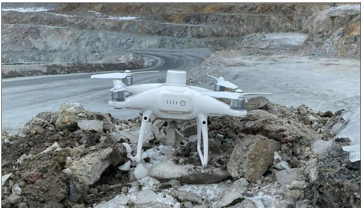
Figure 21. Drone used to collect input photography for the 3D model.
