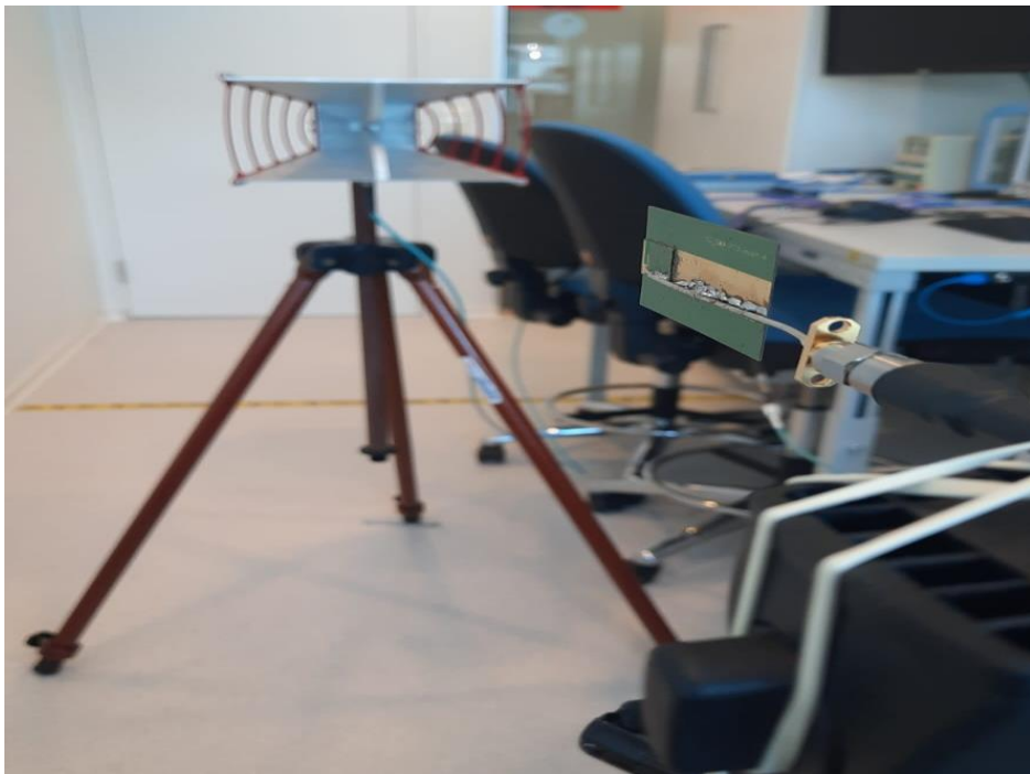
Figure 5.9: Measurement of the designed antenna gain using a horn antenna and Vector Network Analyzer
