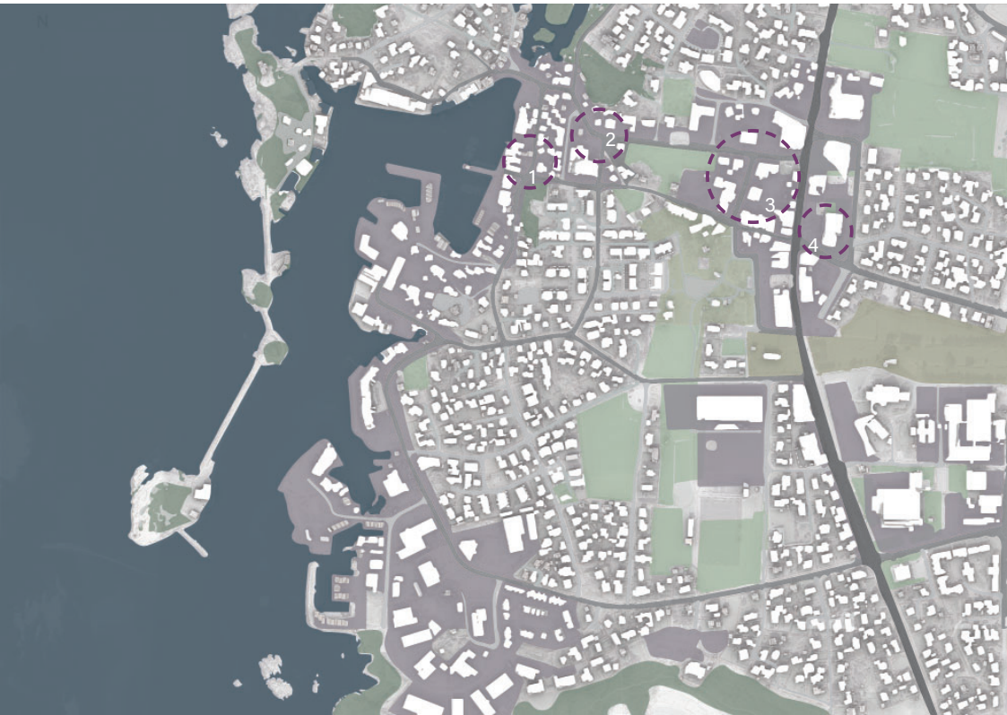
Figure. 37 In this Ground Cover Analysis the Areas of the Development Site with Significant Paved Surfaces That are in Need of Better Drainage Opportunities Have Been Circled.
