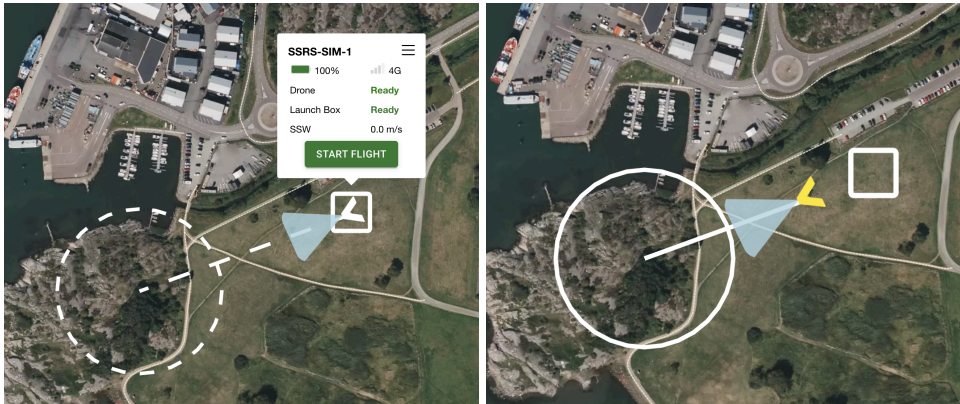
Figure 75. Take off route displayed before pressing “Start Flight” in the final product
