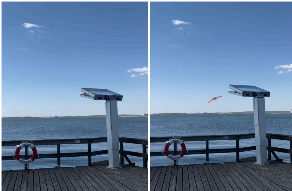
Figure 89. Swedish Sea Rescue Society's drone inside launch box before take off
