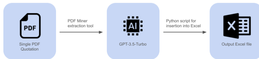
Figure 4.3: Overall architecture of the initial solution
