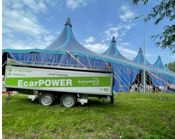
Figure 28. Example of Portable BESS (EcarAccu, n.d)
