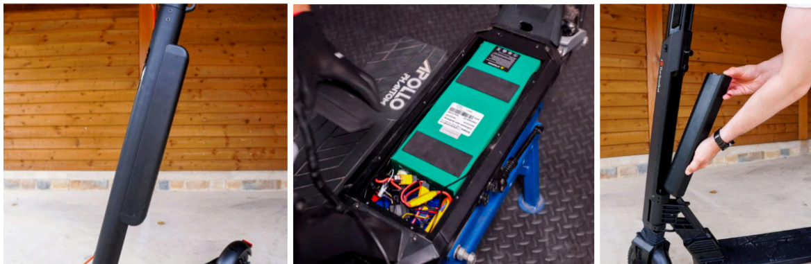
Figure 18. Placements of the battery pack on the electric scooter (Left:Stem, Middle:Deck, Right:Removable) (Frisby, 2023)
