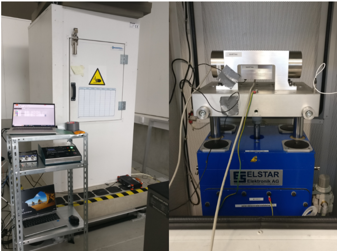
Figure 18: The shock machine Elstar from the outside (left) and on the inside (right). The black duct taped cable leading to the middle weight is the accelerometer for the fixture, while the rightmost white cable connected to the "table" is the accelerometer for the machine. Grey cables goes into the weights in the middle and the left, which lead to the bolts.
