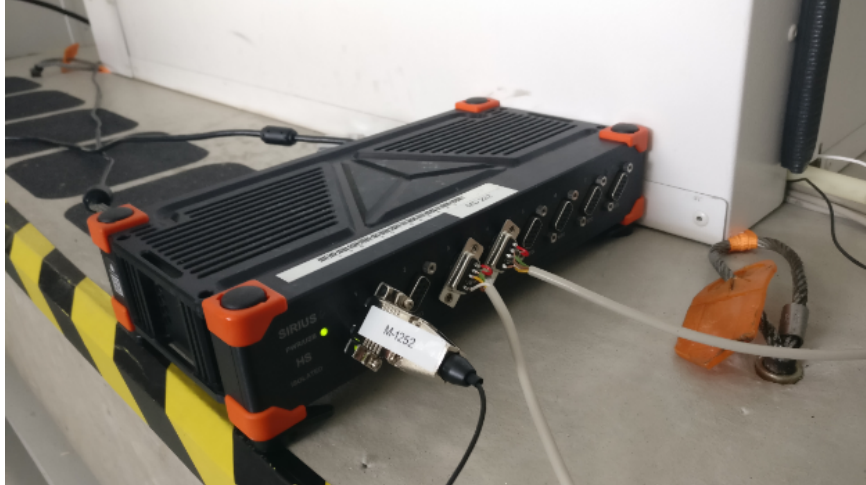
Figure 19: SIRIUSi-HS with the accelerometer in the first channel and the two bolts to be analyzed connected to a channel each, the third and the fourth.
