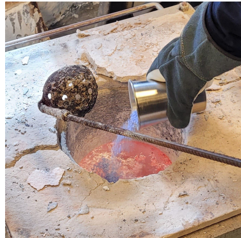
(b) Salt flux being deposited into the melt.
