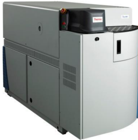
Figure 2.5: Example of apparatus used for optical electron spectroscopy, in image an iSpark 8820 OES Metal Analyzer from Thermo Fischer Scientific [32].
