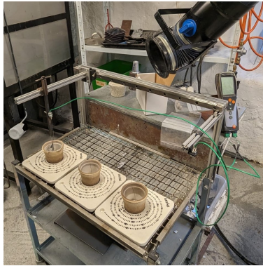
(a) Testing cart with LOOP cartridges placed on mesh shelf.
