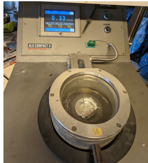
(b) Top view with specimen loaded.
