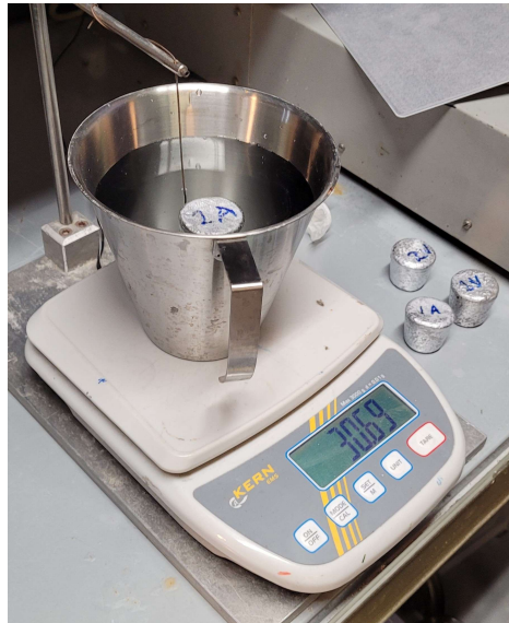
Figure 3.4: Weighing specimen submerged in water. Source: BRYNE AB.
