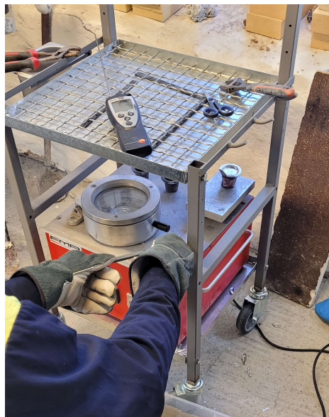
Figure 3.3: Density Index setup. Source: BRYNE AB.
