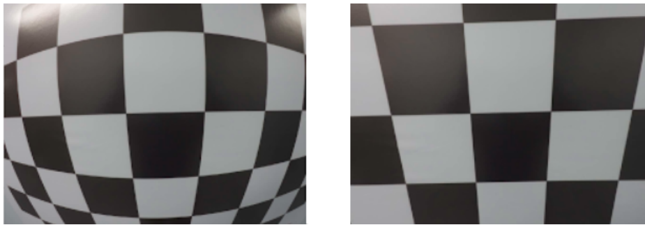
Figure 2.7.1 Original image (on the left) compared to undistorted image (on the right), after correcting lens distortion [21].
