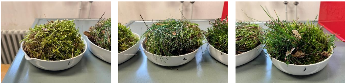
Figure 7: Samples for determining the packing ratio of the considered fuel bed. Photos from BAM.
