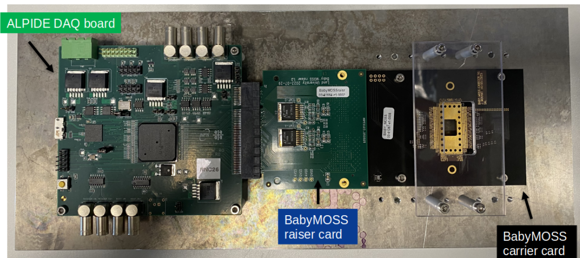
Figure 16. Picture from the author, showing the babyMOSS testing system. It includes the ALPIDE DAQ board, the V1.0 raiser board and the babyMOSS carrier board.
