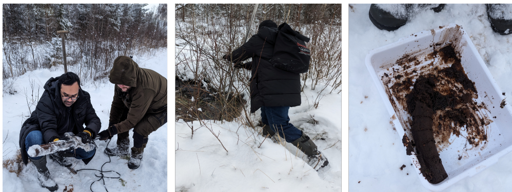
Figure 18: Sample collection process of sediment from R7-D1 ditch. First and second picture is showing sample collection process and third picture is showing collected sediment column. The sampler using in this figure is Kajak Sediment Sampler.
