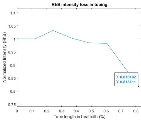
Figure 12. Normalized intensity as a function of the proportion of tubing submerged in the heatbath
