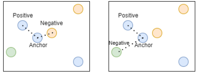
(a) Hard triplet selection : The positive is randomly selected from the blue class and the negative is the closest different class.
